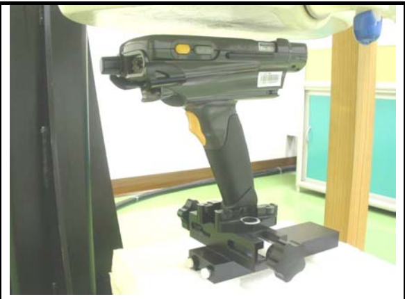
D: EUT with gun in body position The front of the EUT face to the phantom with 15mm-separation distance.
