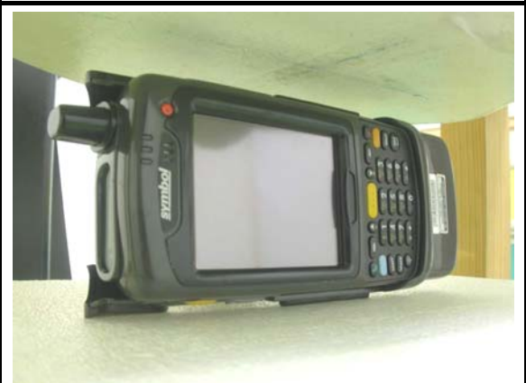
F: EUT with gun in body position The left of the EUT face to the phantom with 15mm-separation distance.
