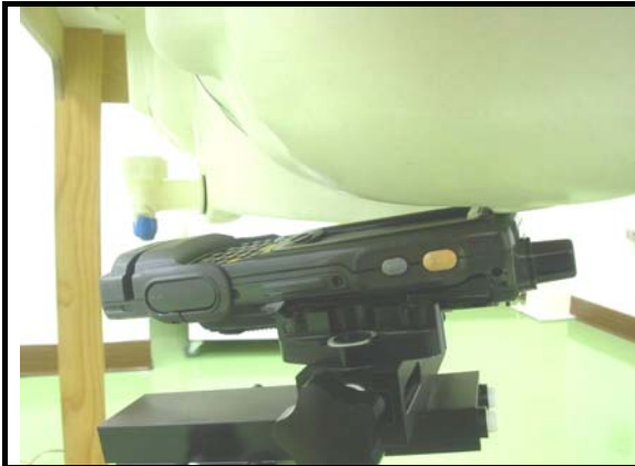
A: EUT with reader in left head tilt position
