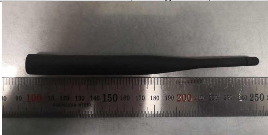
AN2400-P92D01RS (Antenna type: 3.26 dBi)
