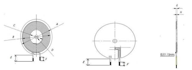
Note: Wrap high-temperature adhesive tape with a width of 8MM (reference) around the outgoing line position of the coil. Stick double-sided adhesive backing on the back of the magnetic sheet.
