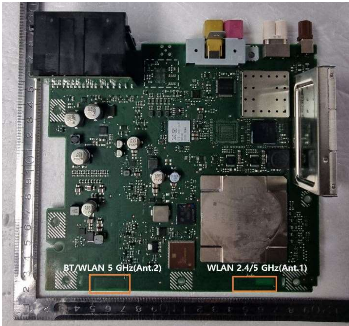
Figure F-1 WLAN Antenna Location
