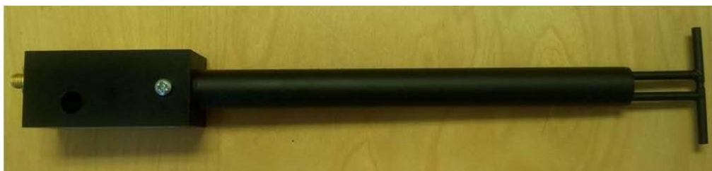
Figure 1 – MVG COMOSAR Validation Dipole
