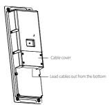
3. Fix the door station and recess bracket.
