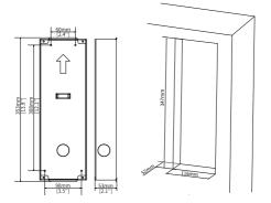
(2) Keep the recess bracket facing outward and upward, and insert four pointed tail cross screws into inside holes to secure the bracket on the wall.
