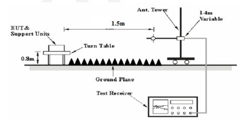
The radiated emission and out of band emission tests use the setup accordance with the ANSI C63.4-2009. The specification used was the FCC 15.209/15.205 and FCC 15.249 limits.
