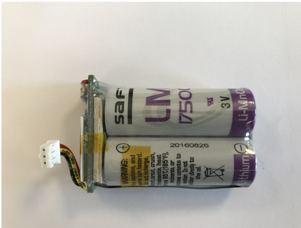
Battery pack with two LM17500 cells (LiMnO 2 /3V).
