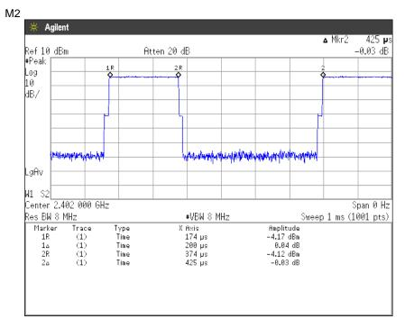
Duty Cycle = Ton / (Ton + Toff) =  $200[\mu s]$  / ( $200[\mu s]$  +  $425[\mu s]$ ) = 32.00[%]
