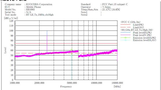
Final Result No. Frequency (P) Reading Reading c.f Result Result Limit AV Result Limit AV Result Limit AV Result AV
