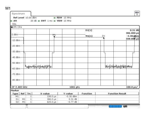
Duty Cycle = Ton / (Ton + Toff) =  $386[\mu s] / (386[\mu s] + 239[\mu s]) = 61.76[\%]$
