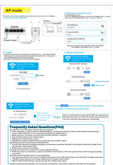
A.If you need reset the extender. You need press and hold the reset button inside the tiny hole for 10 seconds.
