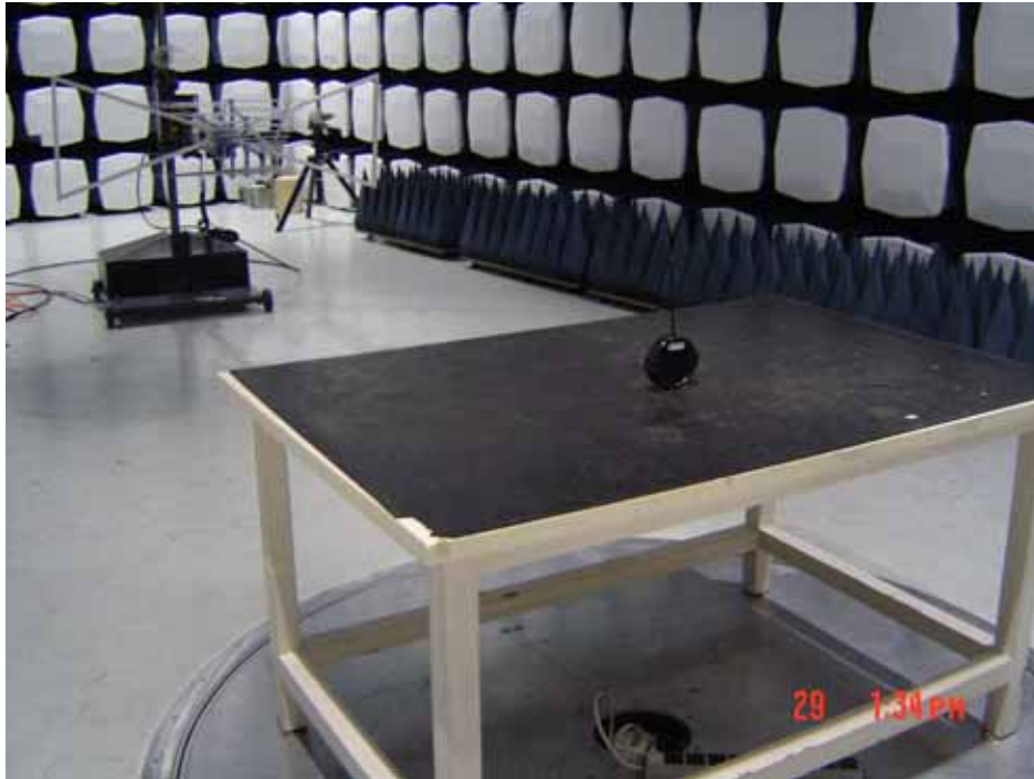
Radiation Emission Test setup
