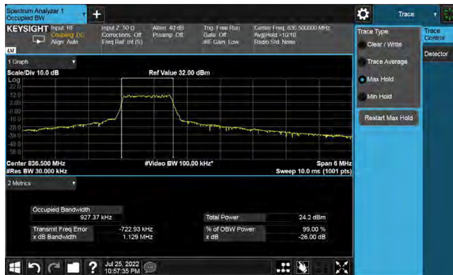
Band26-26dB/99% OBW-26915 Channel-3MHz Bandwidth-16QAM
