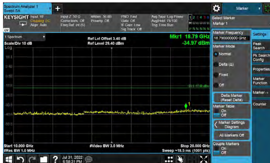
10GHz to 20GHz, Mid Channel, Subcarrier (3.75kHz), QPSK, 1@0
