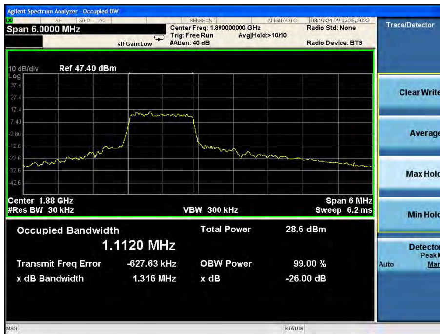
Band2-26dB/99% OBW-3MHz Bandwidth-QPSK
