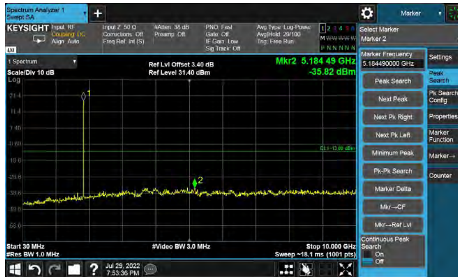
30MHz to 10GHz, Low Channel, Subcarrier (15kHz), QPSK, 1@0
