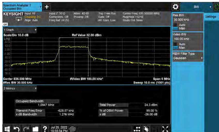
Band26-26dB/99% OBW-26915 Channel-3MHz Bandwidth-QPSK
