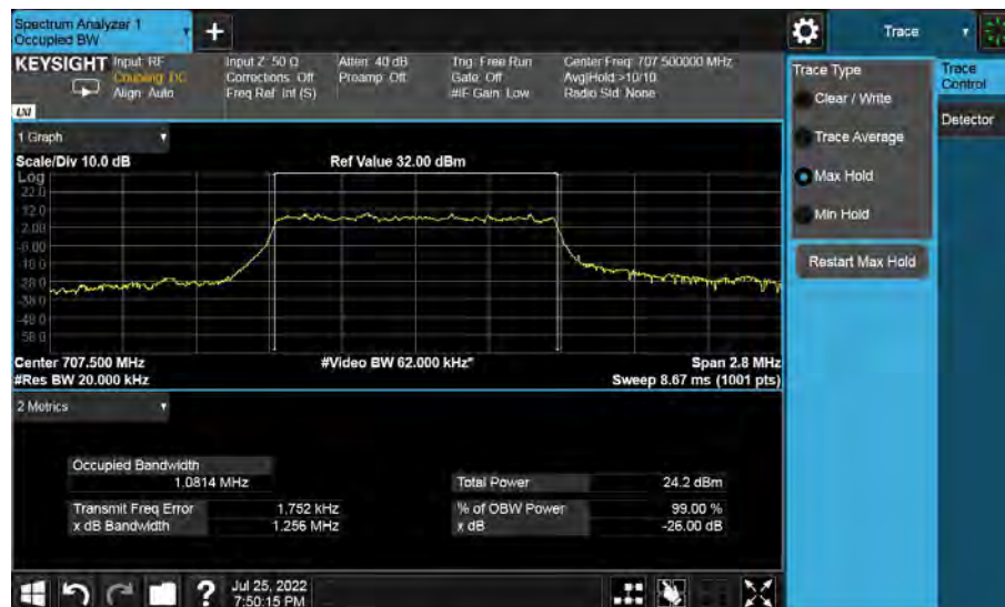
Band12-26dB/99% OBW-1.4MHz Bandwidth-QPSK
