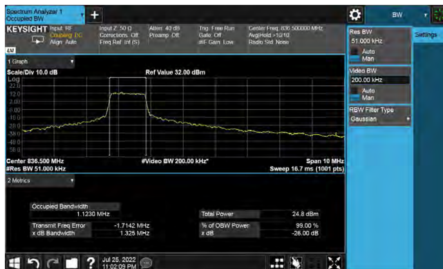
Band26-26dB/99% OBW-26915 Channel-5MHz Bandwidth-QPSK
