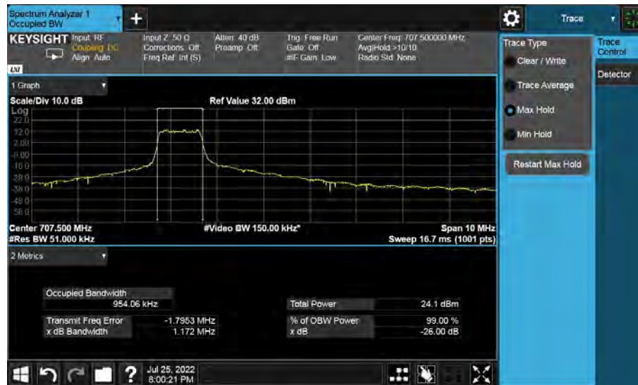
Band12-26dB/99% OBW-5MHz Bandwidth-16QAM
