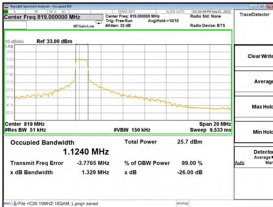
Band26-26dB/99% OBW-26740 Channel-10MHz Bandwidth-QPSK
