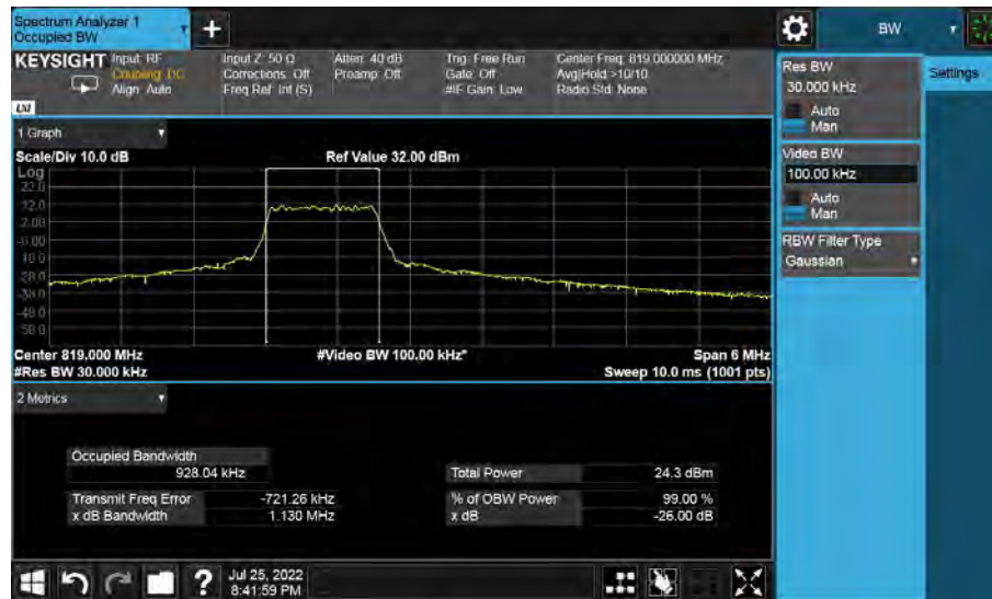
Band26-26dB/99% OBW-26740 Channel-3MHz Bandwidth-16QAM
