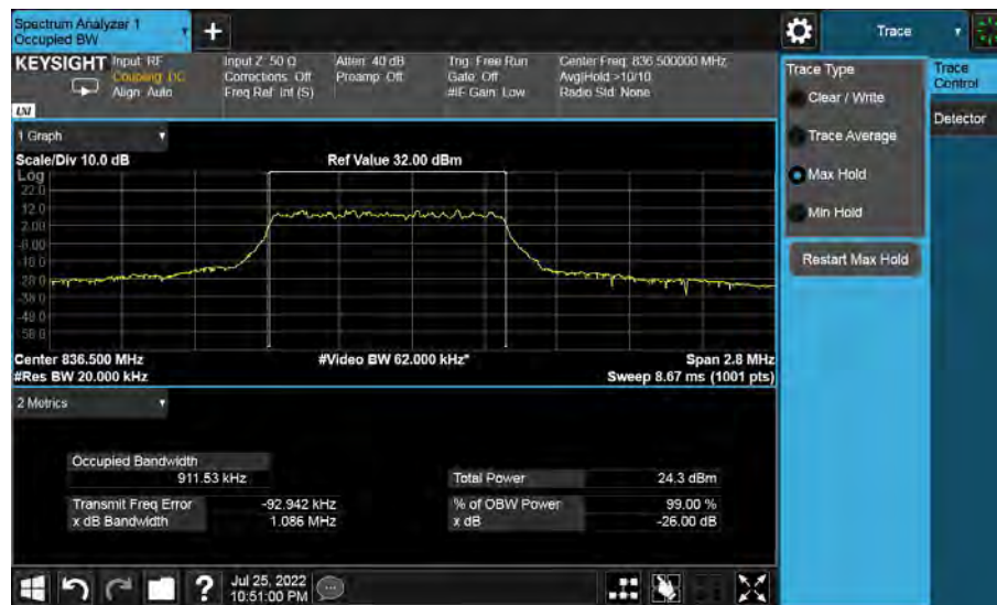
Band26-26dB/99% OBW-26915 Channel-1.4MHz Bandwidth-16QAM
