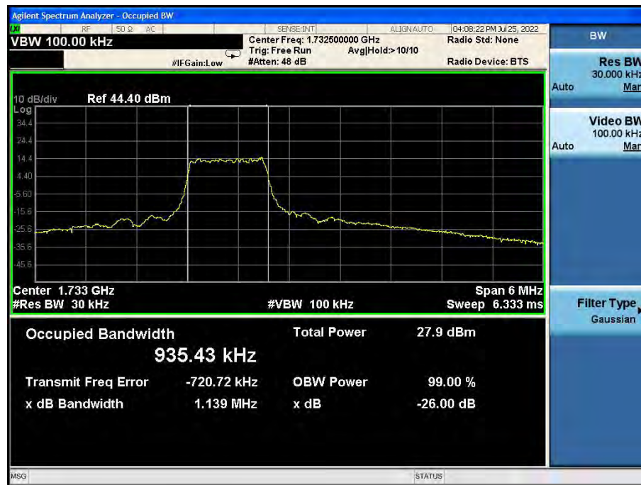
Band4-26dB/99% OBW-3MHz Bandwidth-16QAM
