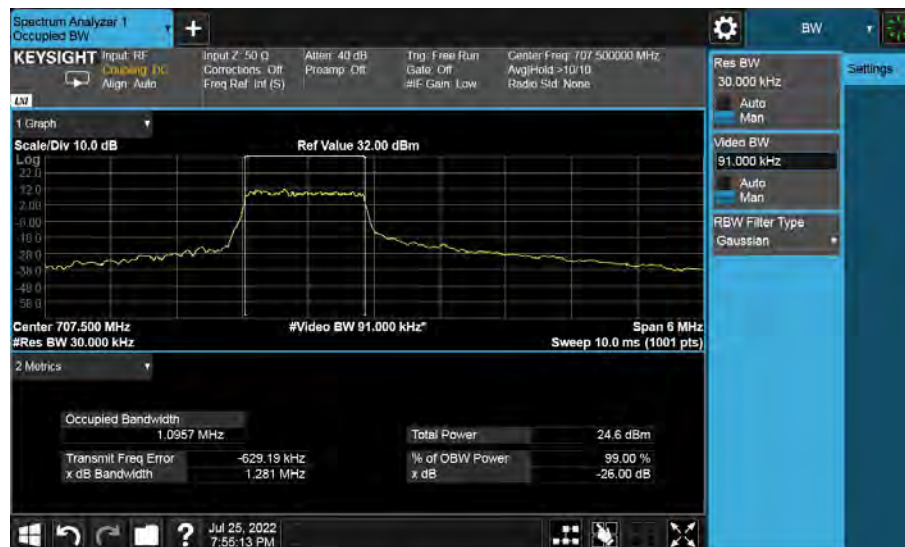
Band12-26dB/99% OBW-3MHz Bandwidth-QPSK
