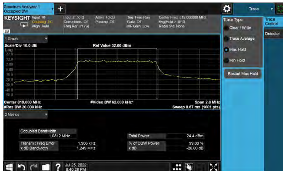
Band26-26dB/99% OBW-26740 Channel-1.4MHz Bandwidth-QPSK
