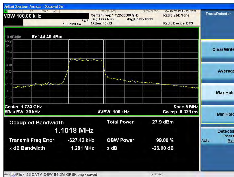
Band4-26dB/99% OBW-3MHz Bandwidth-QPSK
