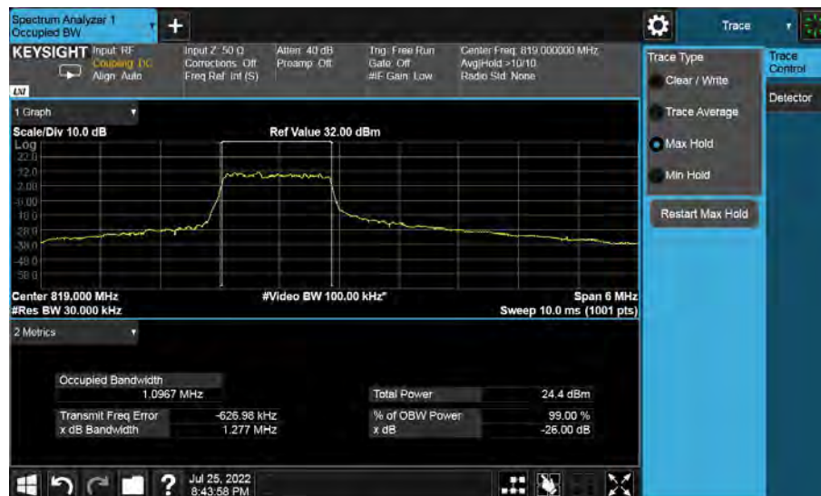
Band26-26dB/99% OBW-26740 Channel-3MHz Bandwidth-QPSK
