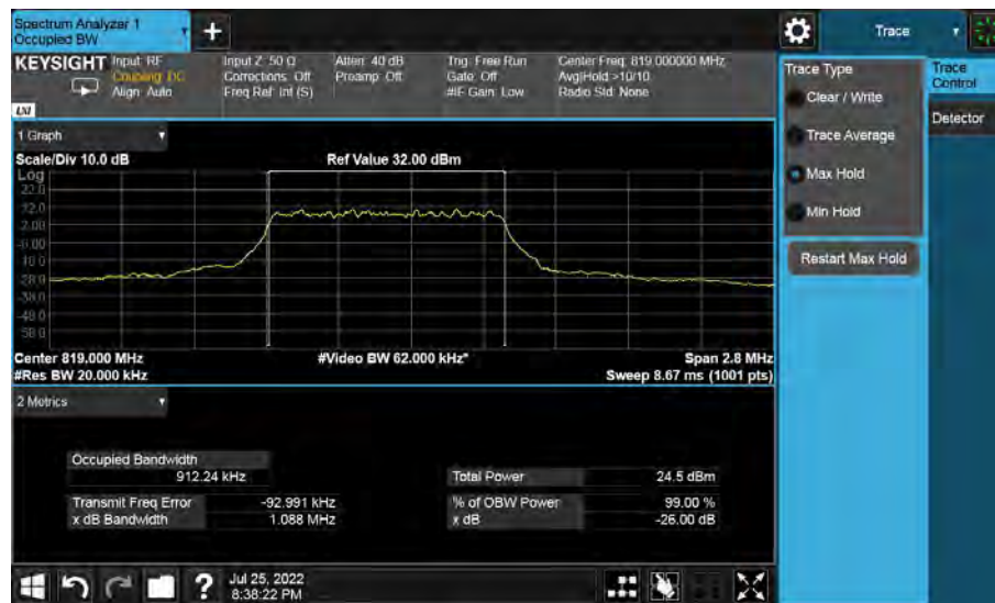
Band26-26dB/99% OBW-26740 Channel-1.4MHz Bandwidth-16QAM
