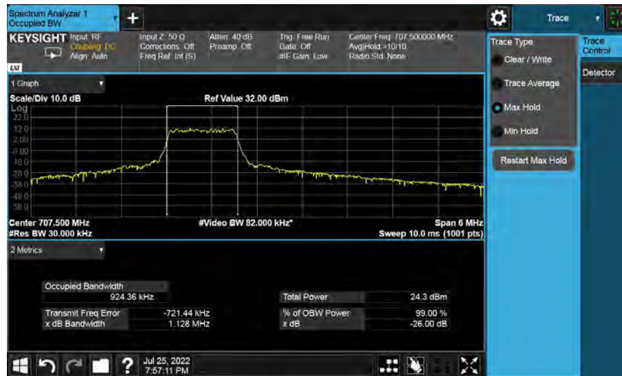
Band12-26dB/99% OBW-3MHz Bandwidth-16QAM
