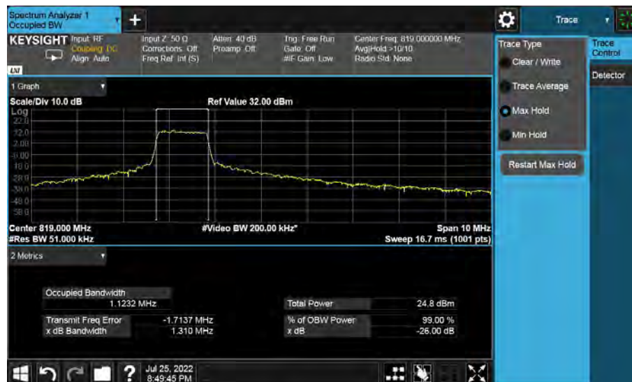
Band26-26dB/99% OBW-26740 Channel-5MHz Bandwidth-QPSK
