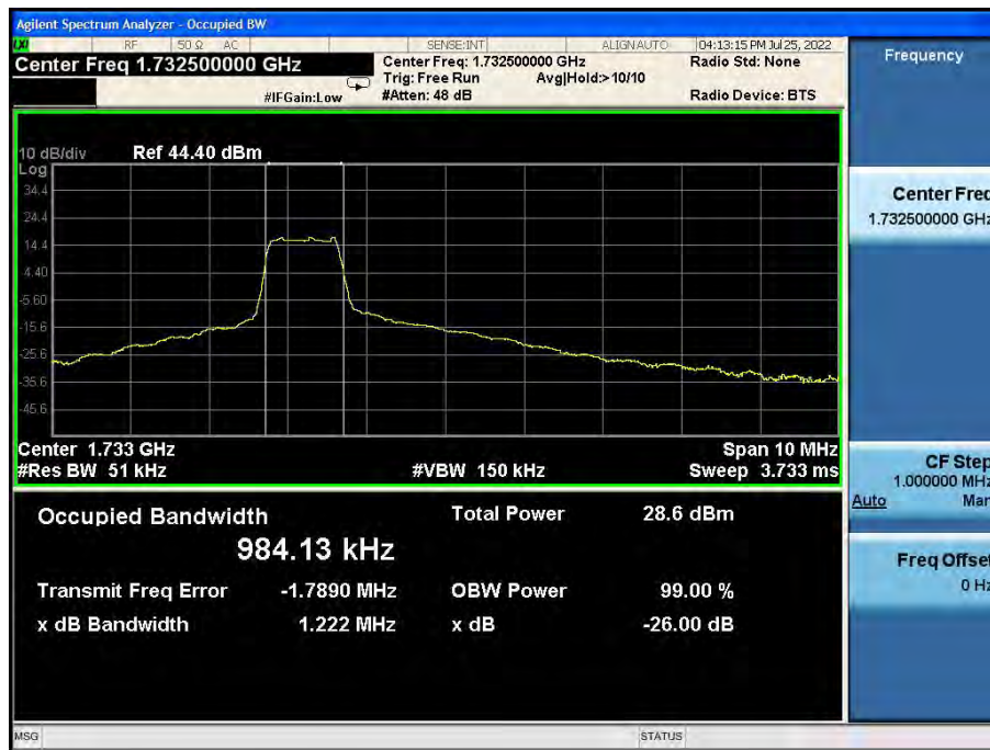
Band4-26dB/99% OBW-5MHz Bandwidth-16QAM
