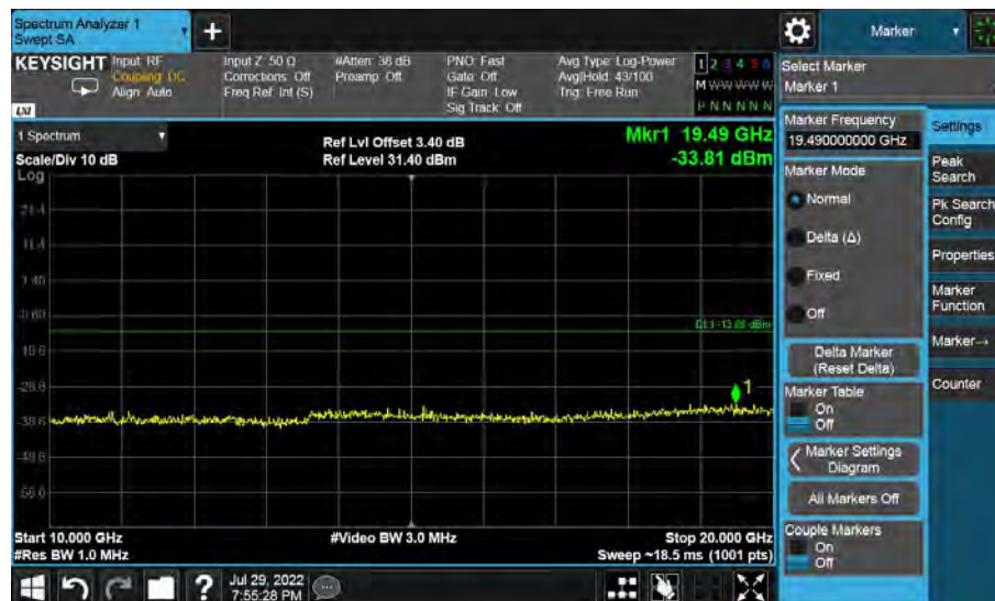
10GHz to 20GHz, High Channel, Subcarrier (15kHz), QPSK, 1@0
