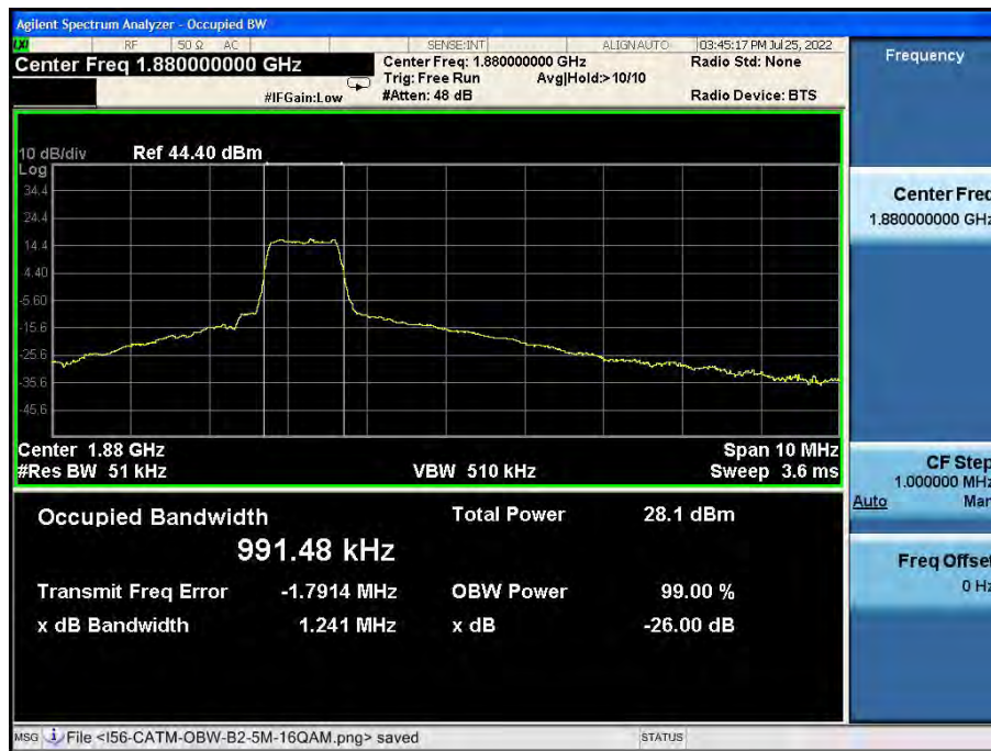
Band2-26dB/99% OBW-5MHz Bandwidth-16QAM
