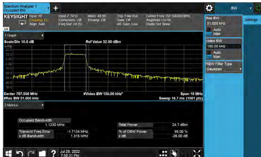
Band12-26dB/99% OBW-5MHz Bandwidth-QPSK
