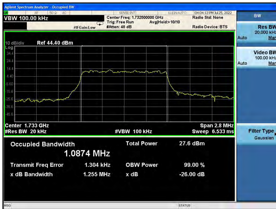
Band4-26dB/99% OBW-1.4MHz Bandwidth-QPSK
