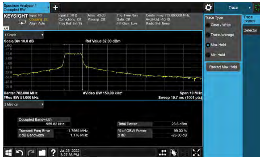
Band13-26dB/99% OBW-5MHz Bandwidth-16QAM
