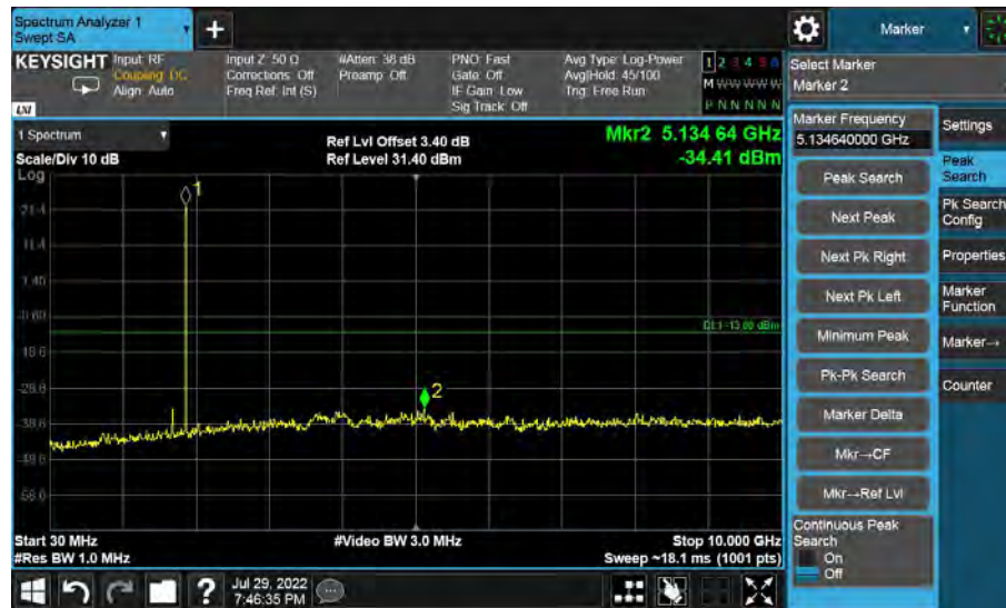
30MHz to 10GHz, Mid Channel, Subcarrier (15kHz), BPSK, 1@0
