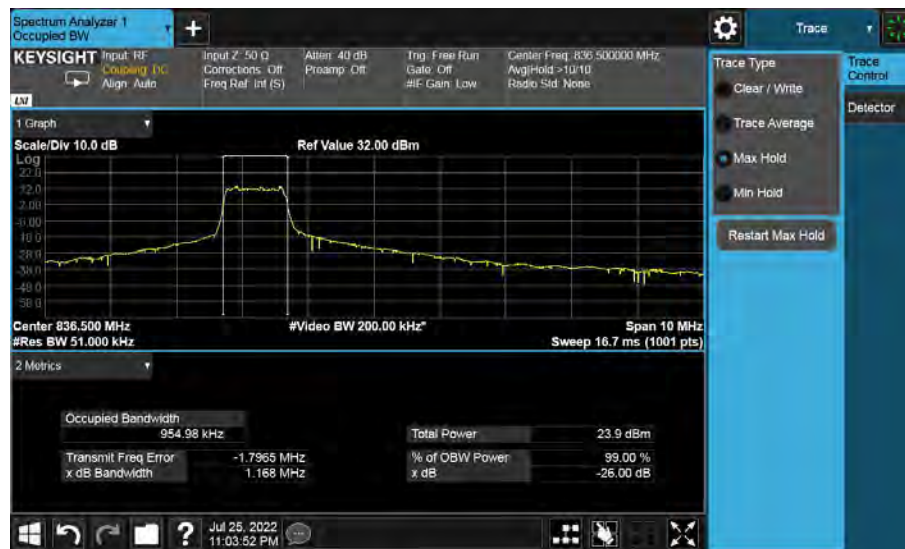
Band26-26dB/99% OBW-26915 Channel-5MHz Bandwidth-16QAM
