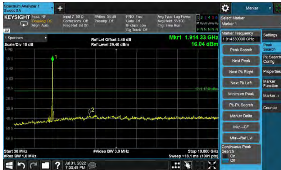
30MHz to 10GHz, High Channel, Subcarrier (3.75kHz), BPSK, 1@0
