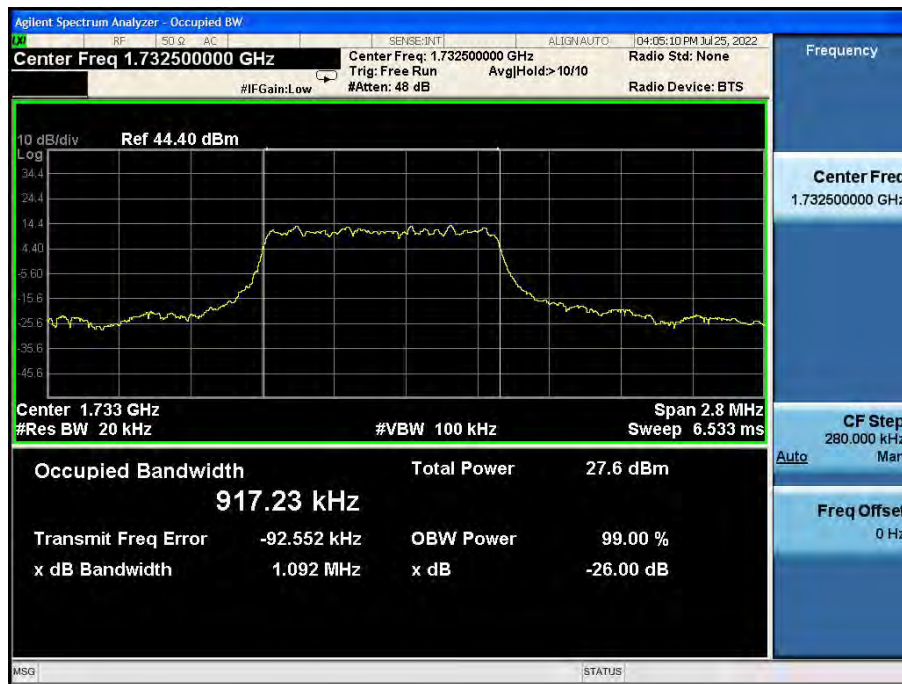
Band4-26dB/99% OBW-1.4MHz Bandwidth-16QAM
