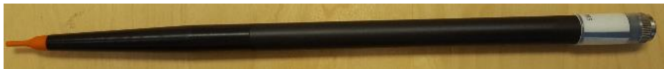
Figure 1 – MVG COMOSAR Dosimetric E field Dipole
