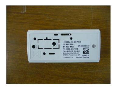
Photograph No.3 Wireless magnetic contact PGP9303 P9M3 Antenna assembly
