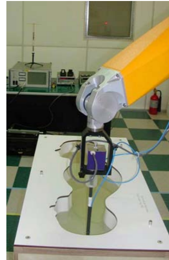
Figure 4. Photograph of the probe and the Phantom
