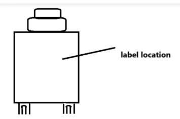
The label is laser onto the surface of the product.
