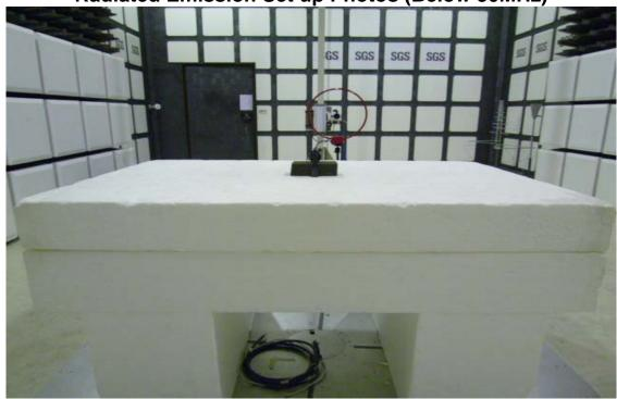
Radiated Emission Set up Photos (Below 1GHz)
