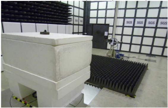
Radiated Emission Set up Photos (Front View)
