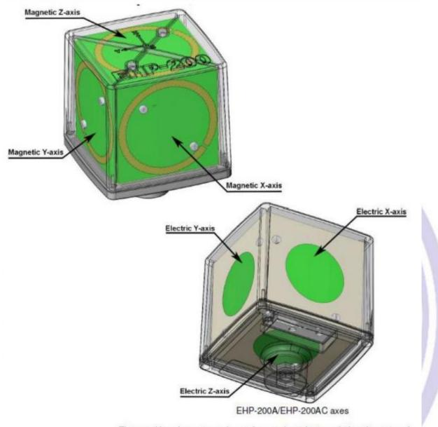
The sensitive elements are located approximately 8 mm below the external surface
