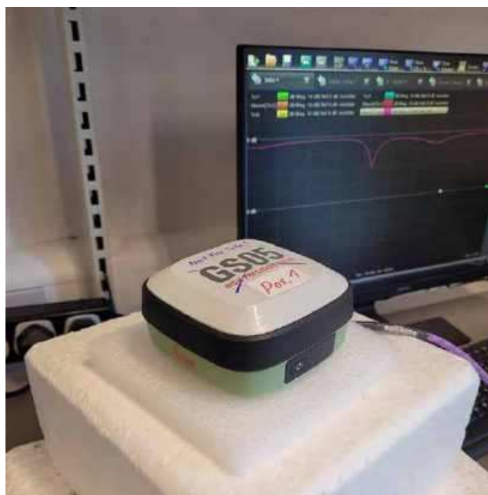
Figure 3 Test Setup for VNA Measurements
