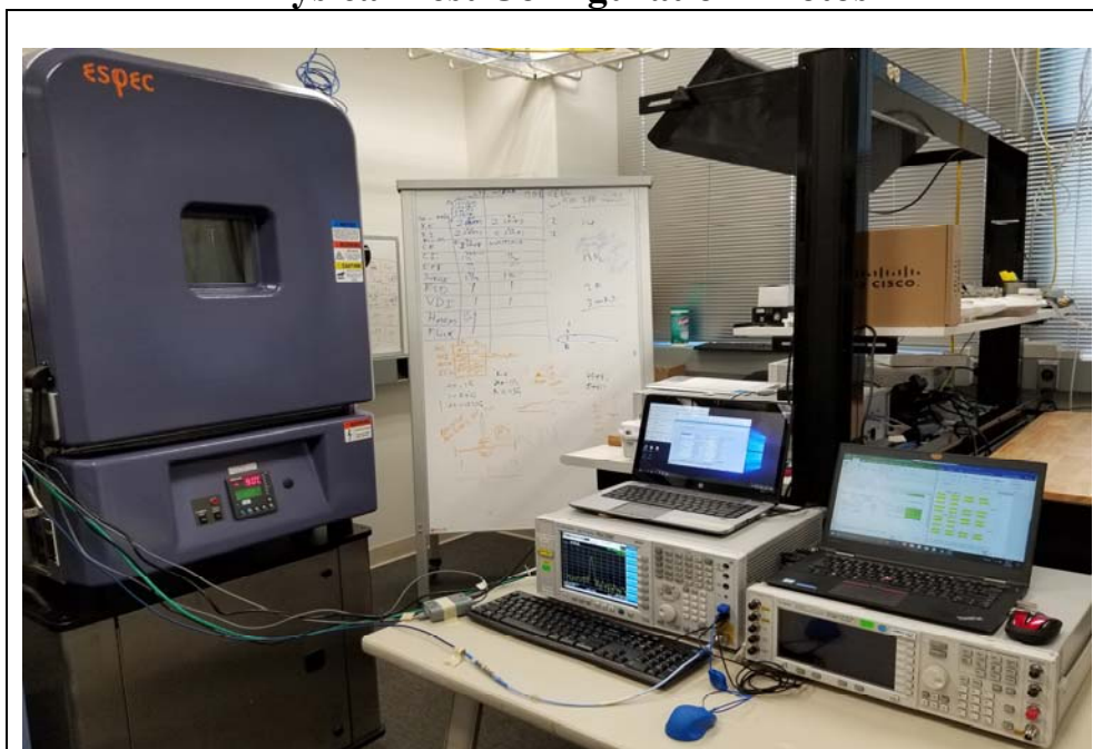
Title: RF Conducted Emissions Test Set Up
