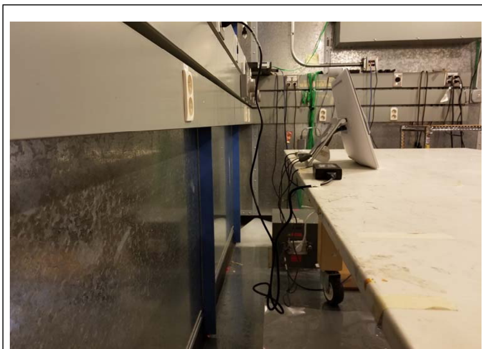
Title: AC Conducted Emissions Test Set Up
