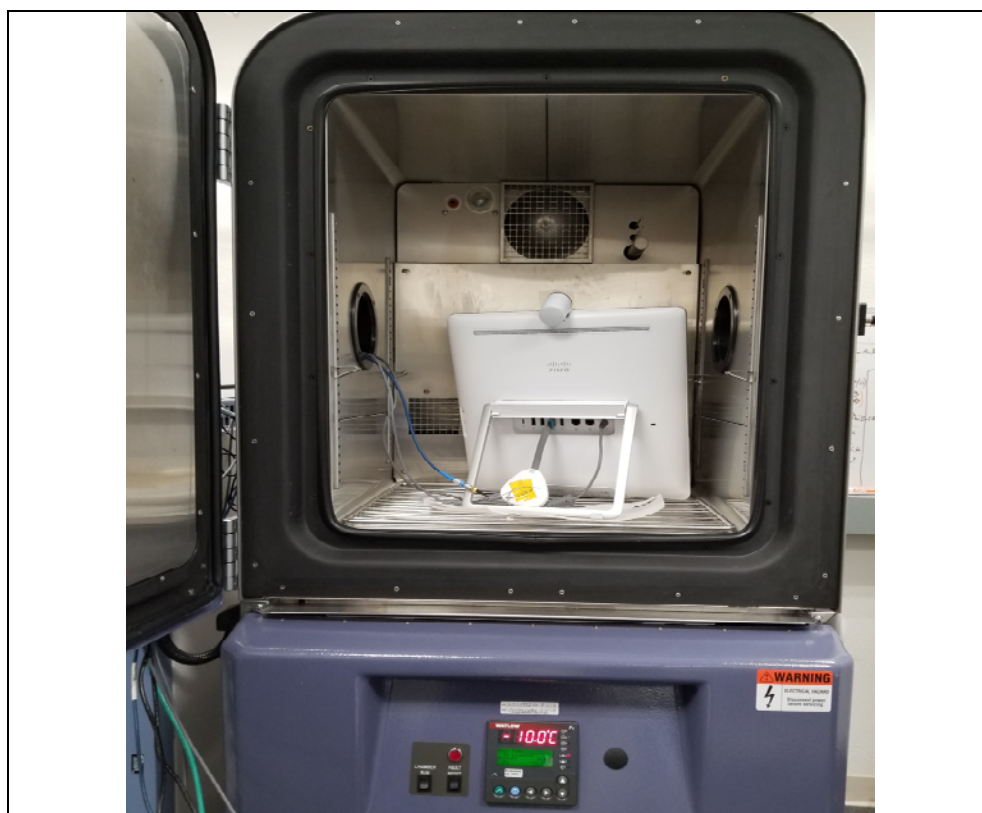
Title: RF Conducted Emissions Test Set Up
