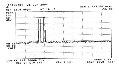
TX<sub>ON</sub> duration after pressing a key and keeping this key pressed!
