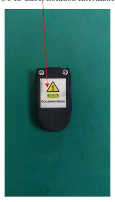
The label shown shall be permanently affixed at a conspicuous location on the device and be readily visible to the user at the time purchase (Labeling requirements per 2.925)
