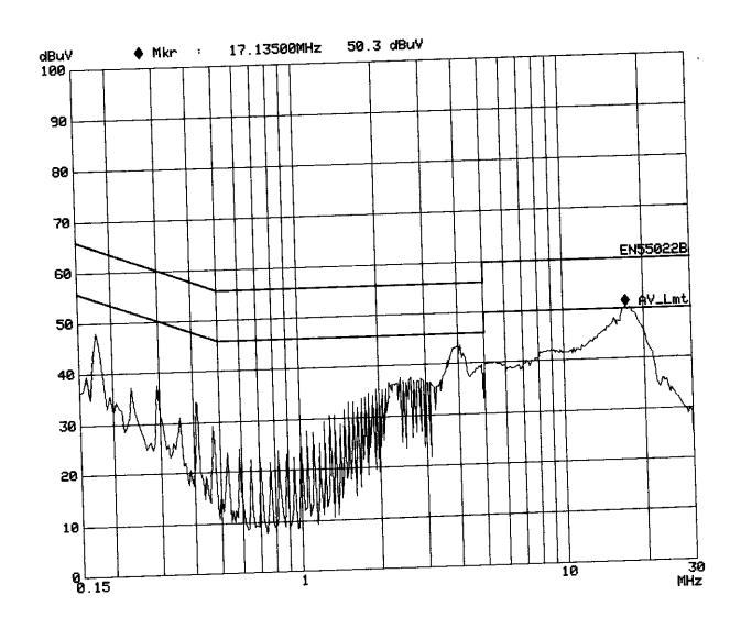
C&C Lab. Conduction Test Site 3 EN55022 Class B
