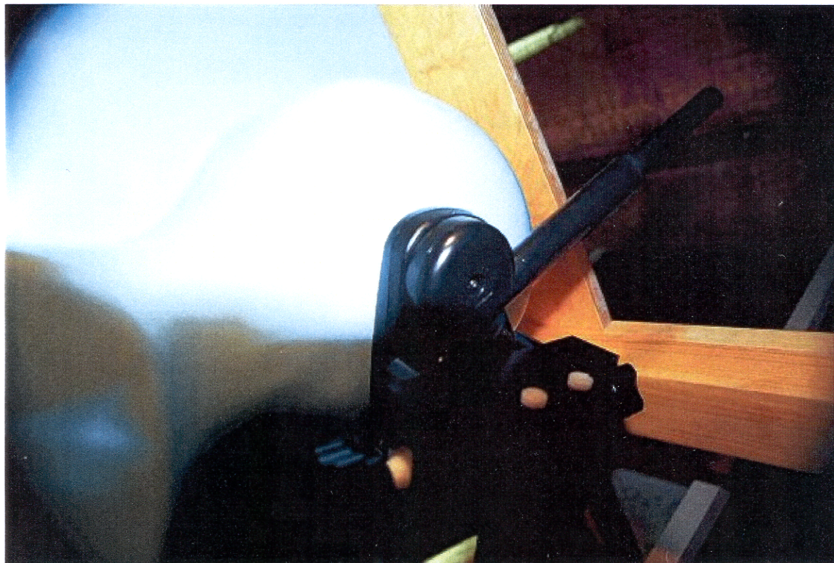
Photo 7 - SAR set-up: Bottom view, right side of head, correct antenna position
