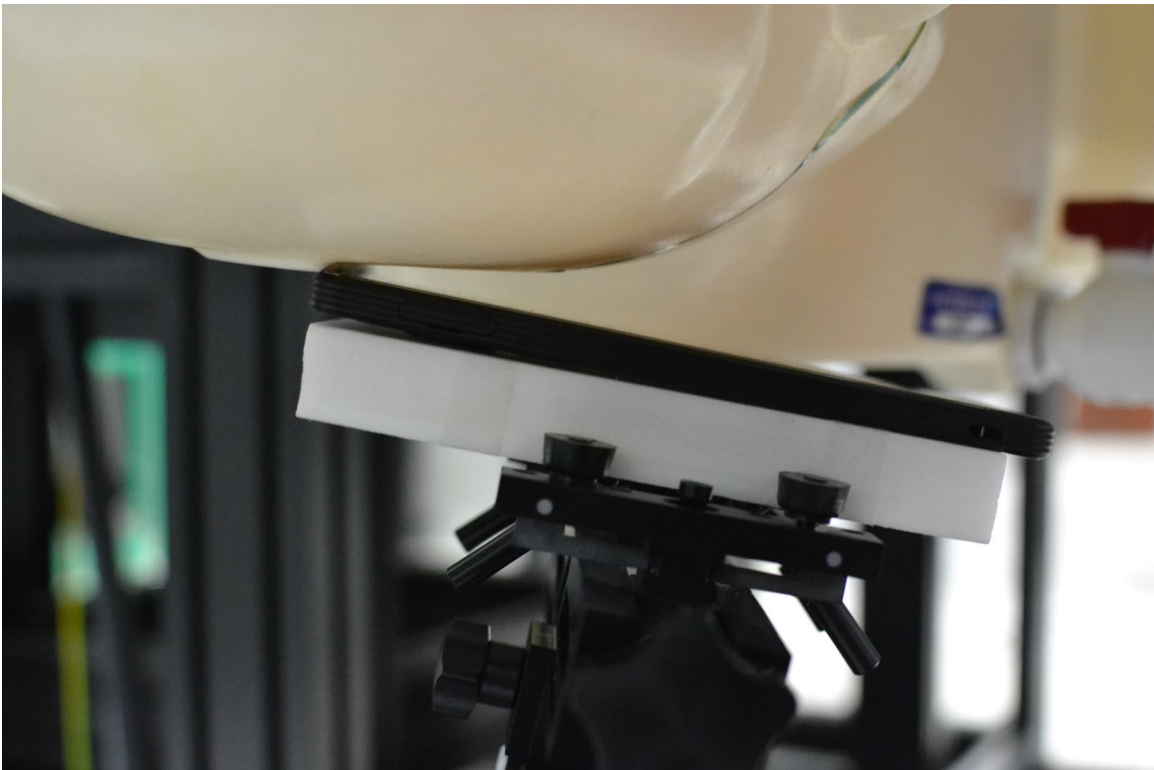
SAR Test Setup Photo 2 – Head, Right Tilt, 0 mm
