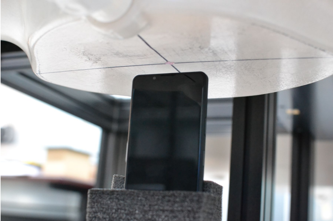
SAR Test Setup Photo 9 – Hotspot, Top Edge, 10 mm
