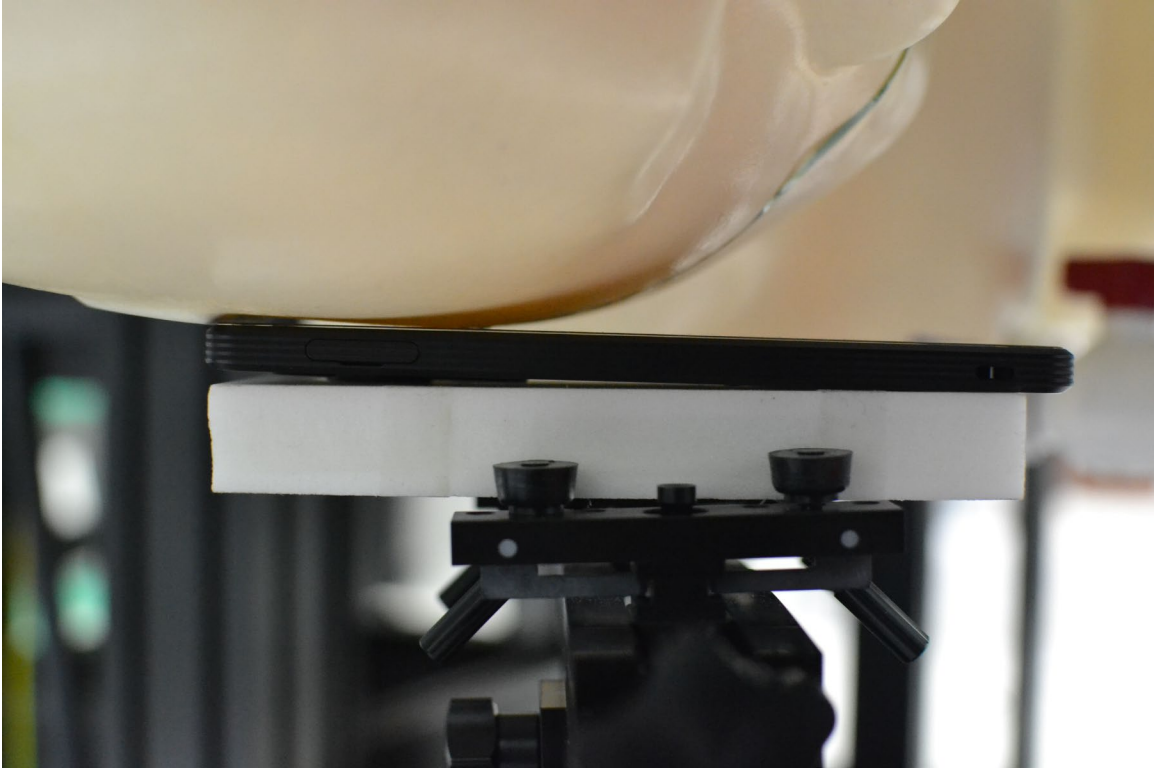
SAR Test Setup Photo 1 – Head, Right Cheek, 0 mm
