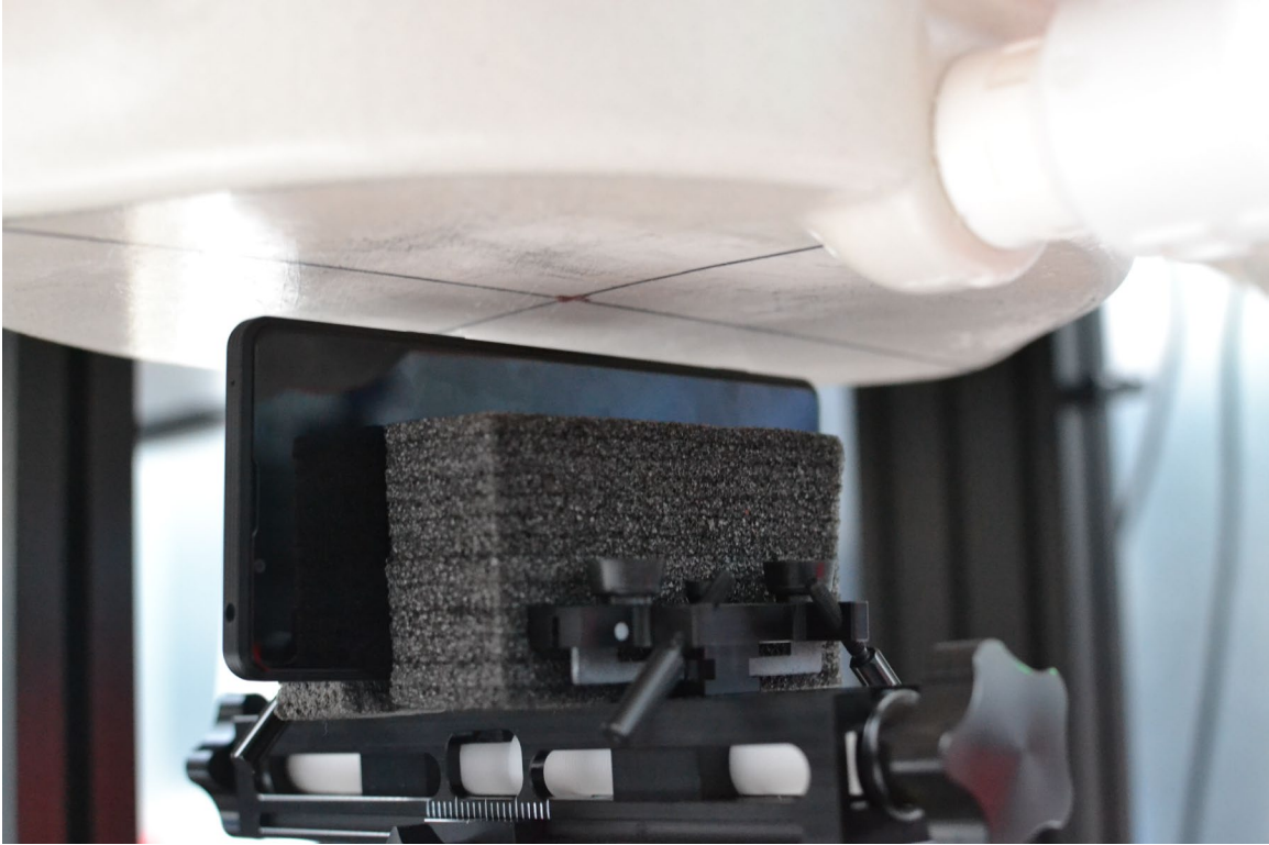
SAR Test Setup Photo 13 – Hotspot, Right Edge, 10 mm
