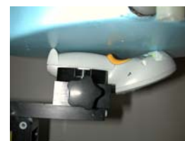
Figure 17. Body SAR Test Setup
