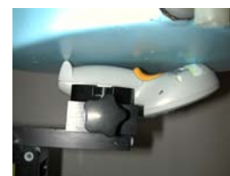
Figure 19. Hand SAR Test Setup
