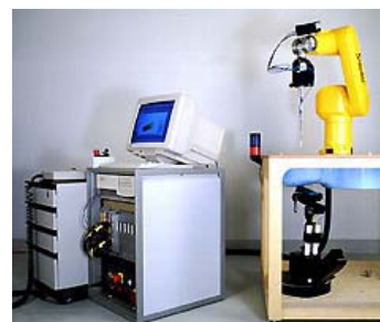
Fig. 1 SAR Test Setup
