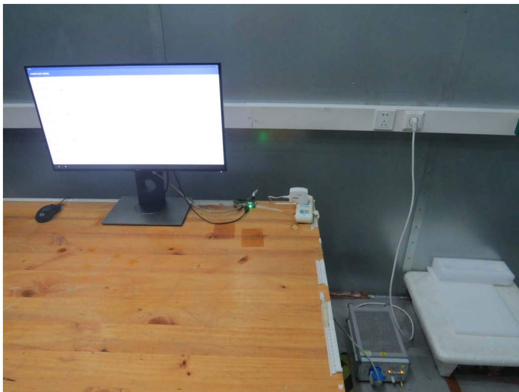
Picture 2 Conducted Emission Test Setup
