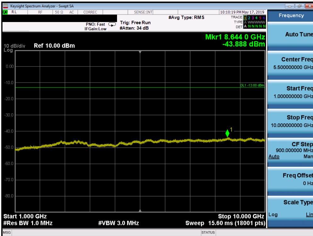
Plot 7-117. Conducted Spurious Plot (Band 13 - 5.0MHz QPSK - RB Size 1, RB Offset 0 - Mid Channel)
