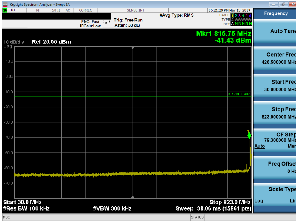
Plot 7-121. Conducted Spurious Plot (Band 26/5 - 10.0MHz QPSK - RB Size 1, RB Offset 0 - Low Channel)
