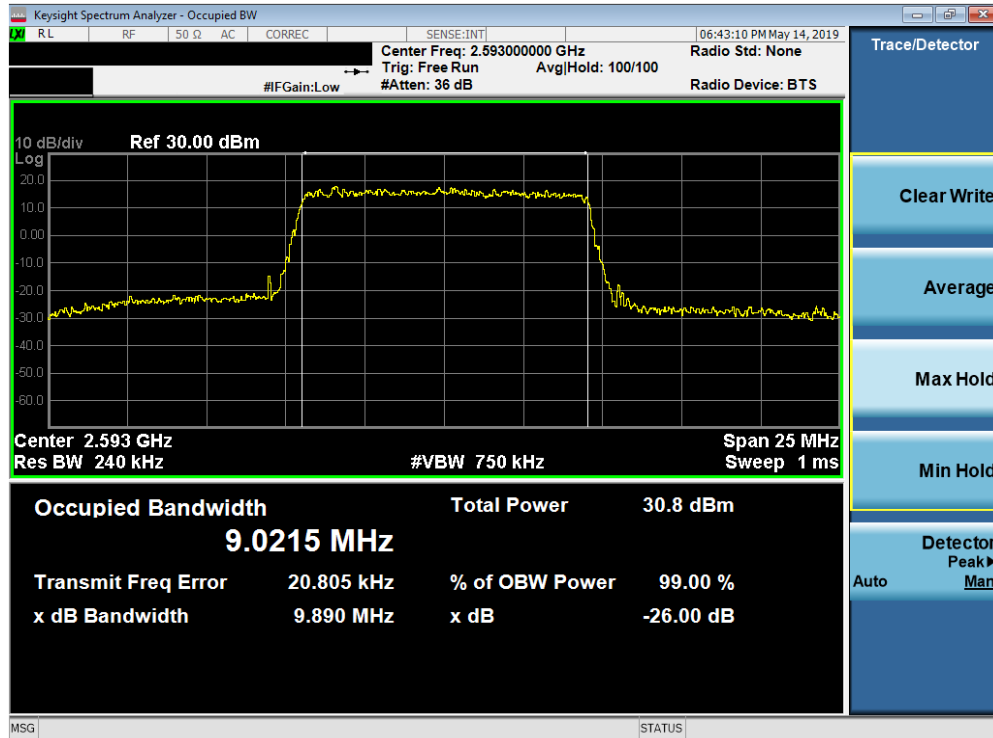
Plot 7-86. Occupied Bandwidth Plot (Band 41 - 10.0MHz 16-QAM - Full RB Configuration)
