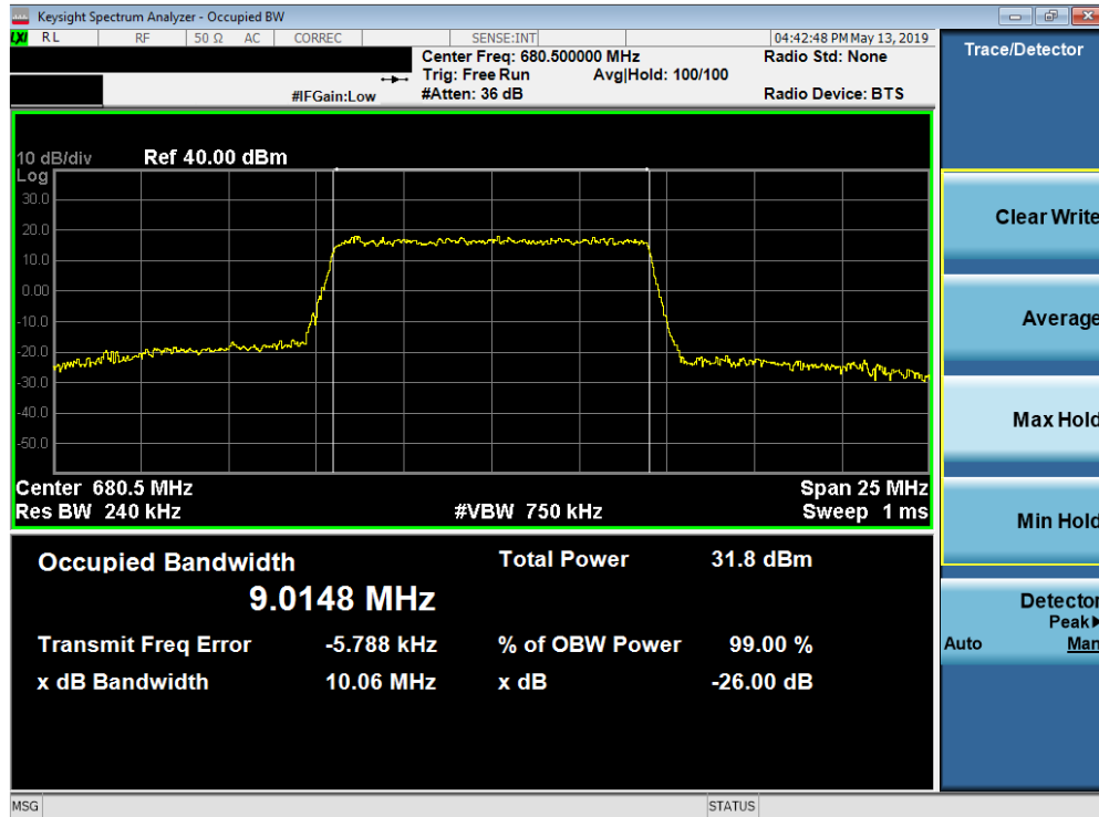
Plot 7-5. Occupied Bandwidth Plot (Band 71 - 10.0MHz 16-QAM - Full RB Configuration)
