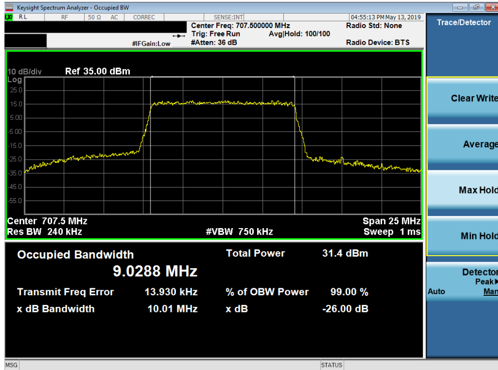
Plot 7-23. Occupied Bandwidth Plot (Band 12/17 - 10.0MHz 16-QAM - Full RB Configuration)
