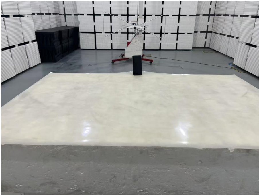
Set-up for Radiated Spurious Emission, Above 1GHz
