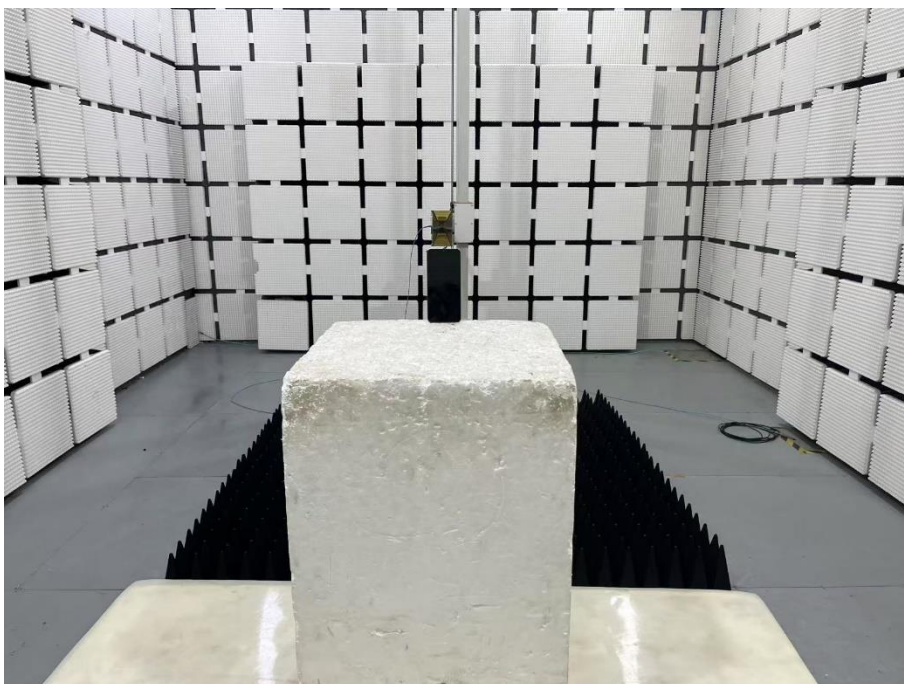
Set-up for Radiated Spurious Emission, Above 1GHz
