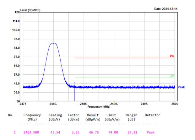
Project No.: 2403Z107562E-RF Tester: Mack Huang Condition: PK trace RBW:1MHz; VBW:3MHz; SWT:0.3sec Polarization: Horizontal Note: BLE 2Mbps Low Channel 2402MHz
