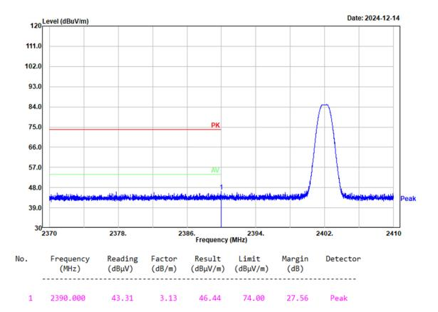
Project No.: 2403Z107562E-RF Tester: Mack Huang Condition: PK trace RBW:1MHz; VBW:3MHz; SWT:0.3sec Polarization: Vertical Note: BLE 1Mbps Low Channel 2402MHz
