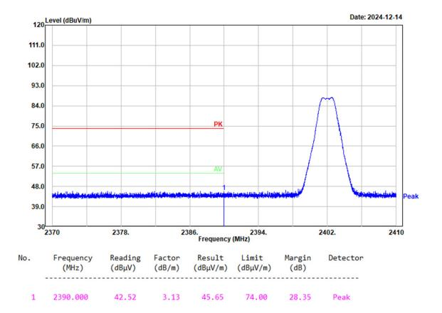
Project No.: 2403Z107562E-RF Tester: Mack Huang Condition: PK trace RBW:1MHz; VBW:3MHz; SWT:0.3sec Polarization: Horizontal Note: BLE 2Mbps High Channel 2480MHz
