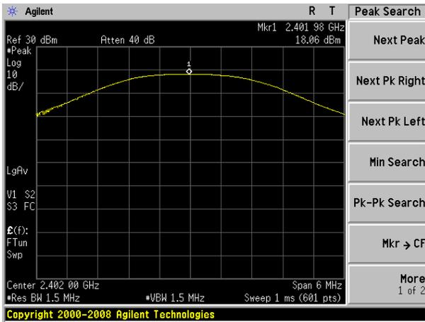
Peak output Power plot on channel 39 (3Mbps)
