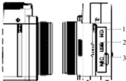
1. HD TV Port: Connects to high-definition display devices for high-quality audio & video transmission.
