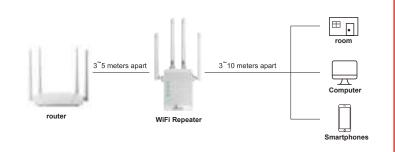
When installing, the WiFi repeater should be installed next to the router or in a place with a strong signal; After installation, the WiFi Repeater should oe placed 3~6 meters away from the router
