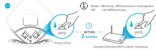
Press the **WPS** button once, the WX3310-B1 WPS LED (3) blinks green. Within Two minutes, press the WPS button on your modem/router. Then the WiFi LED 🤝 blinks slowly (1 sec on and 1 sec off) during setup. If the WX3310-B1 WPS LED 🕔 turns red, do the
