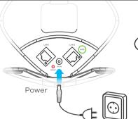
Green Blinking - System is booting. On - System is ready.
