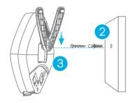
Place the WX3310-B1 so the wall mount hole lines up with the screw. Slide the WX3310-B1 down gently to fix it into place.
