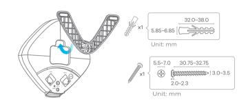
Attach the bracket to the back of the WX3310-B1 as shown.
