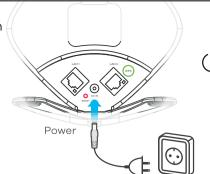
Green Blinking - System is booting. On - System is ready.
