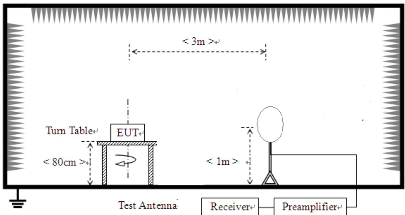
For radiated emissions from 30MHz to 1GHz
