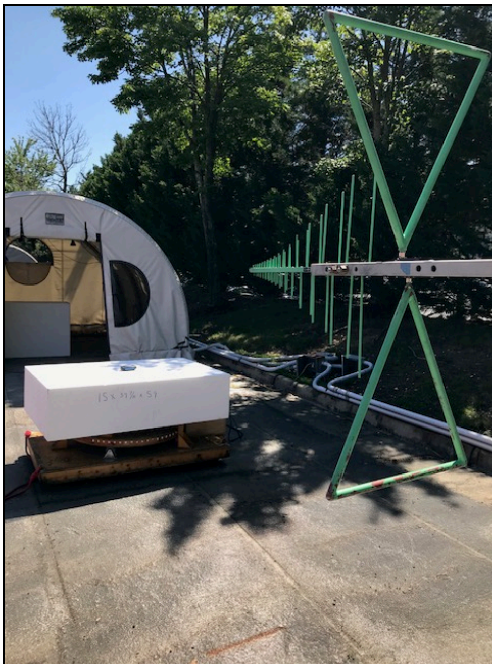
Photograph 1: Radiated Emissions Testing– NFC 30 MHz to 1 GHz – Front View
