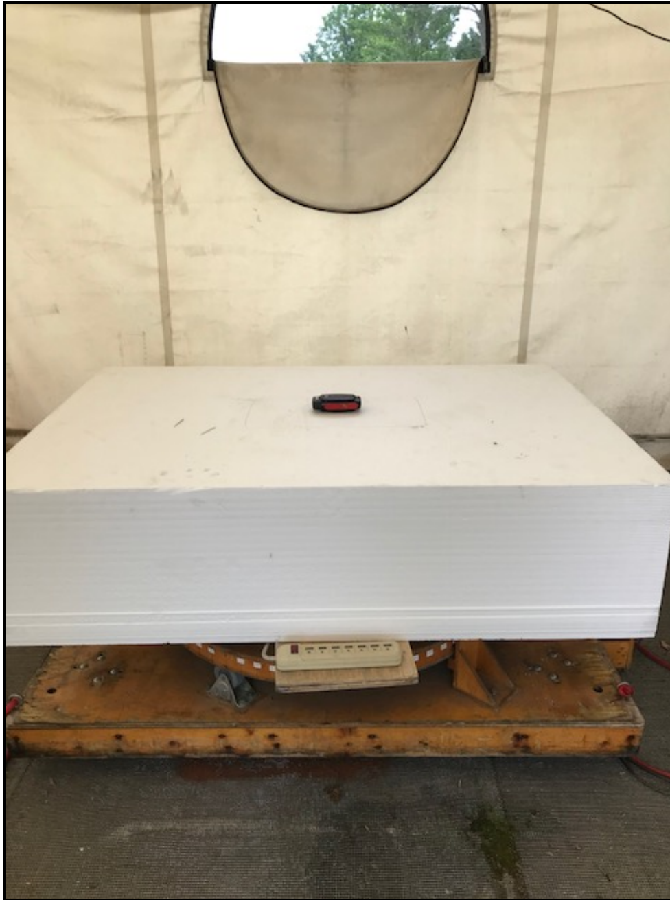
Photograph 3: Radiated Emissions Testing – NFC 9 kHz to 30 MHz – Front View
