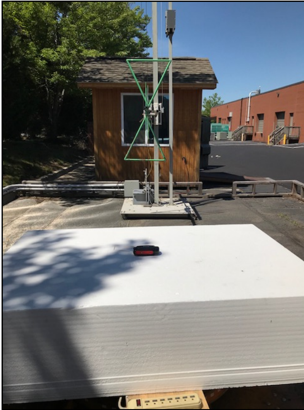
Photograph 2: Radiated Emissions Testing – NFC 30 MHz to 1 GHz – Back View
