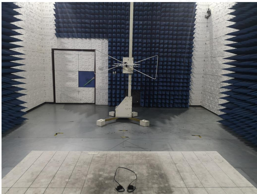
RADIATED EMISSION TEST SETUP ABOVE 1GHZ
