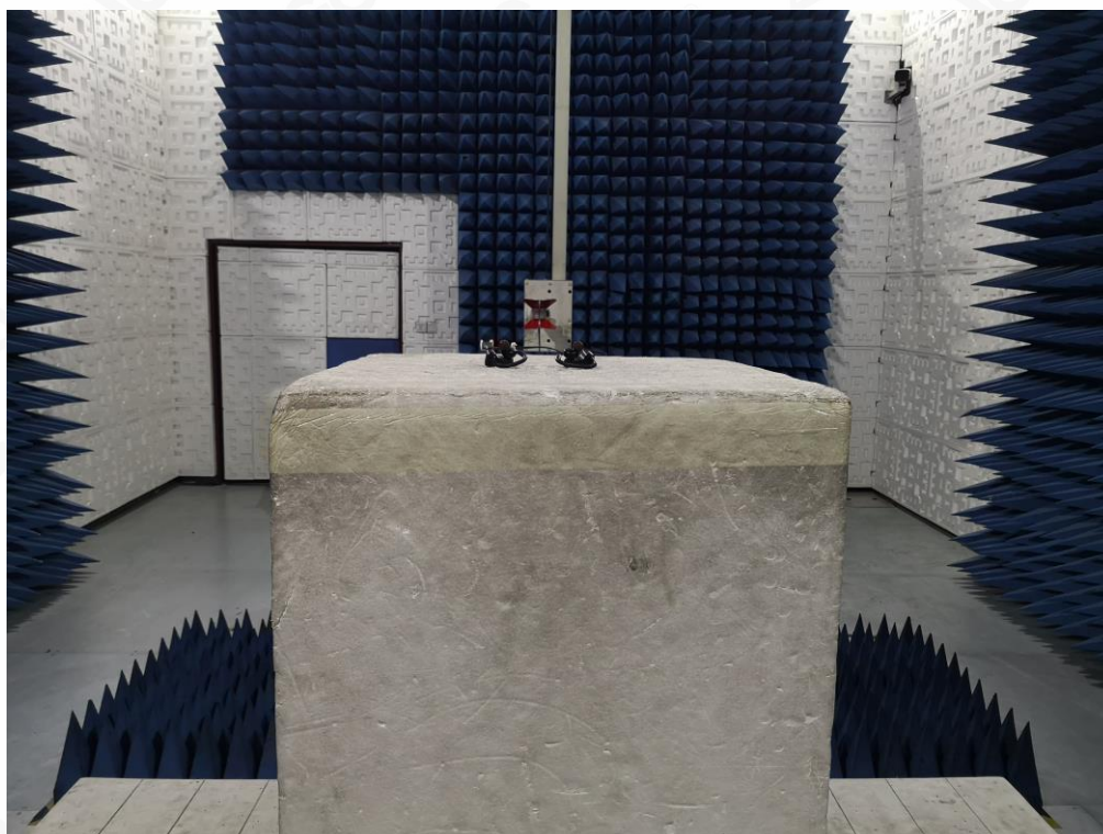
RADIATED EMISSION TEST SETUP ABOVE 1GHZ
