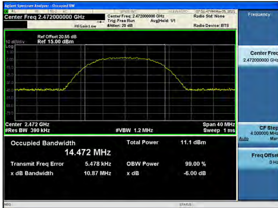
99% Bandwidth plot (802.11b-CH 13)
