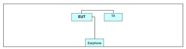
Non-Conductive Table Power Line: 120 VAC, 60 Hz
