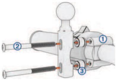
**NOTE:** Both  $^{1}/_{4}$  in. standard and M6 bolts are included. Match the size of the factory bolts on your clutch-clamp or brake-clamp bracket.
