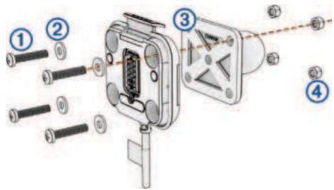
2 Tighten the nuts 4 to secure the base plate.
