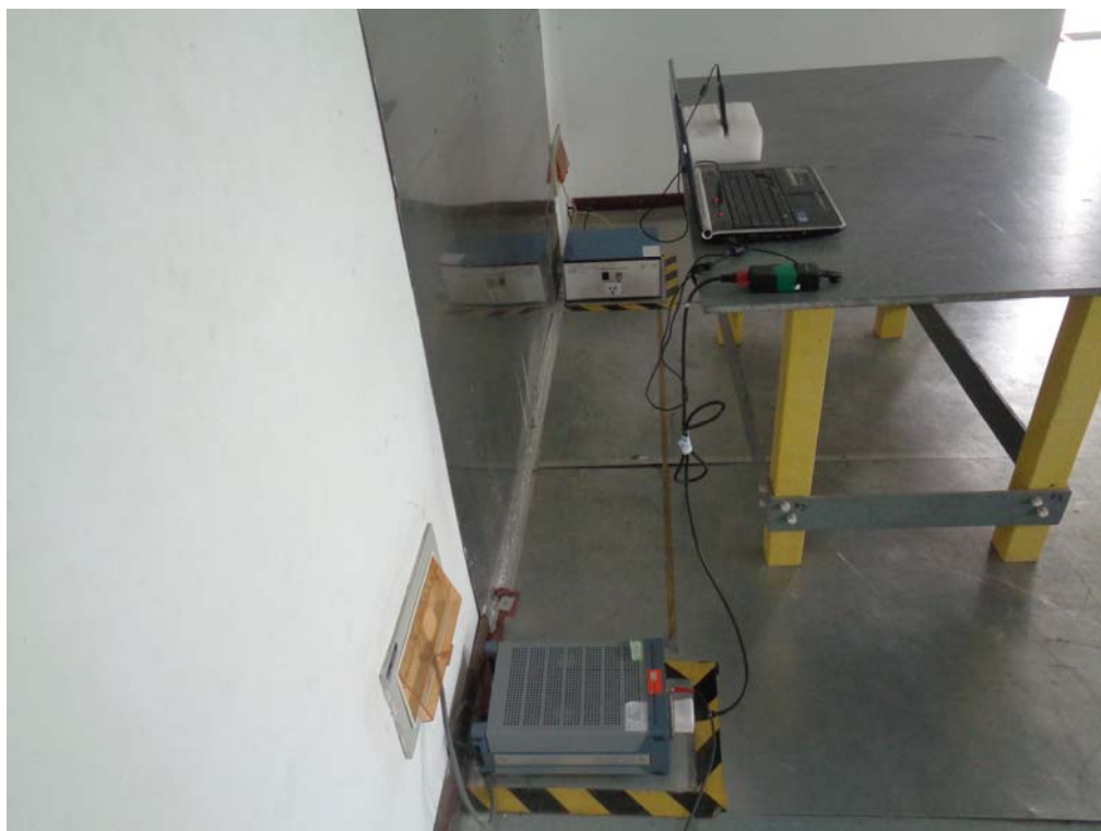
Conducted Emissions Test Setup Side View
