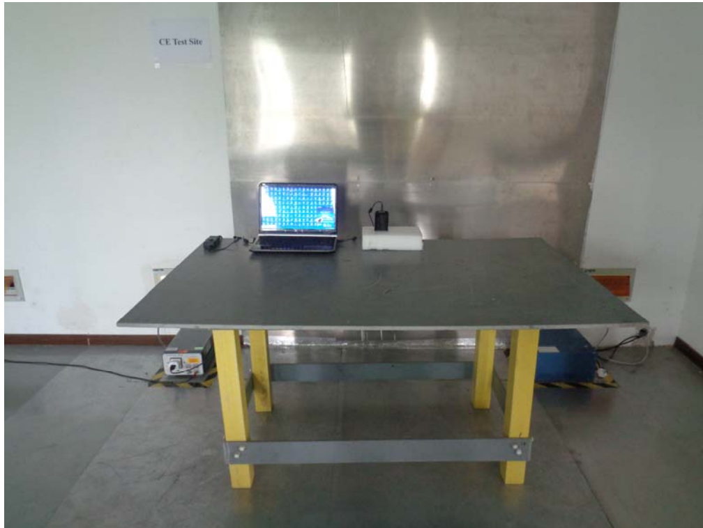
Conducted Emissions Test Setup Front View
