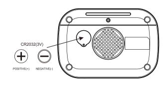
The lithium backup battery needs replacement when the LOW BATTERY indicator flashes, otherwise, the time and alarm settings will be lost/reset
