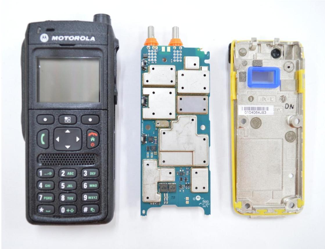
RF Board with Chassis and Housing (Front Side), Model MTP3550
