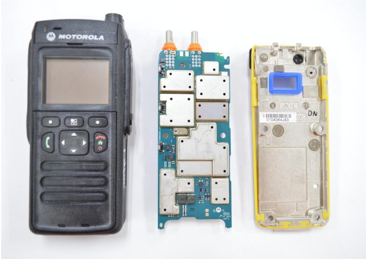
RF board with Chassis and Housing (Front Side), Model MTP3500
