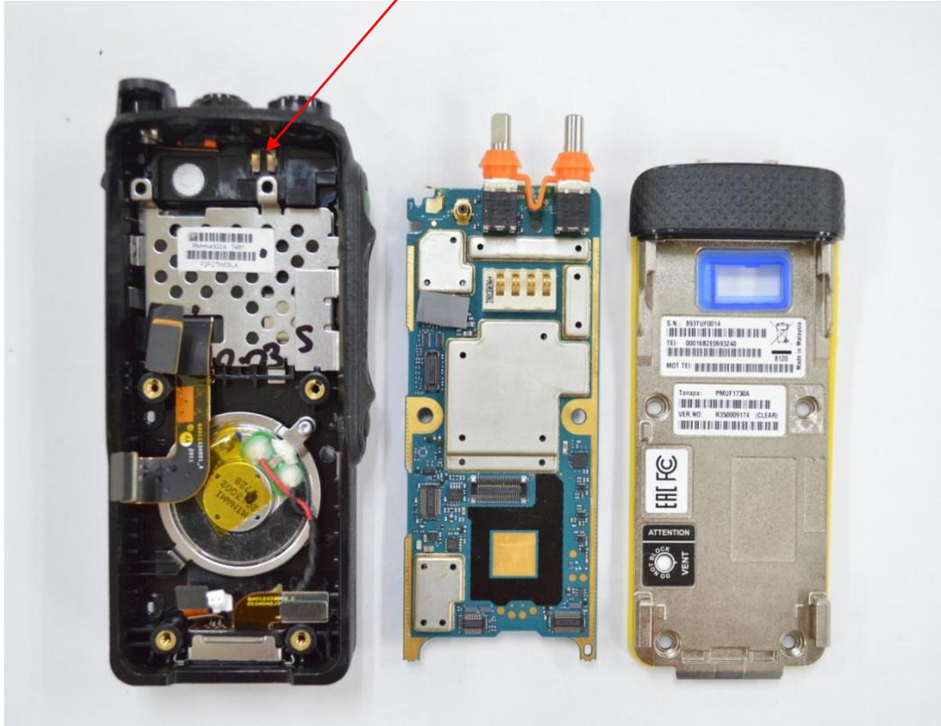
RF Board with Chassis and Housing (Back Side), Model MTP3550 / MTP3500
