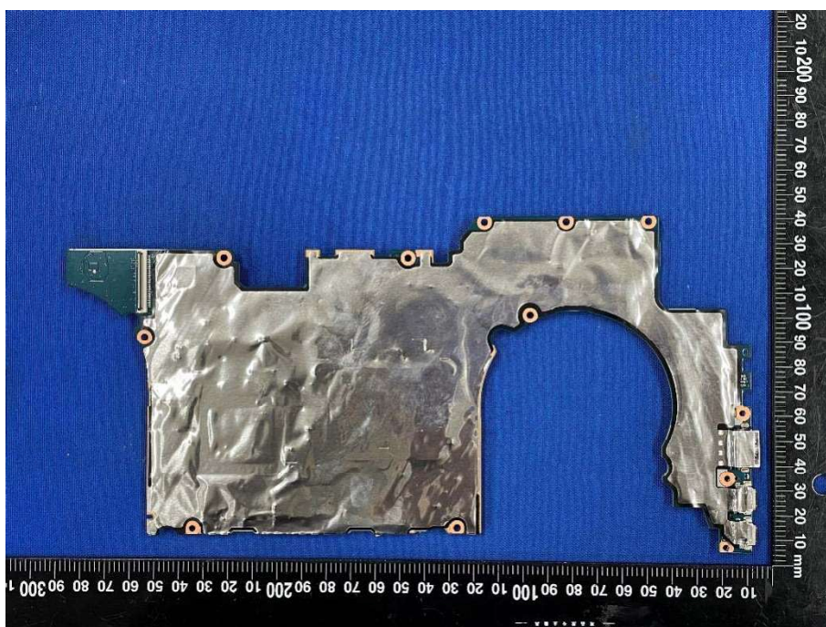
MAIN BOARD REAR VIEW (WITH SHIELDING)
