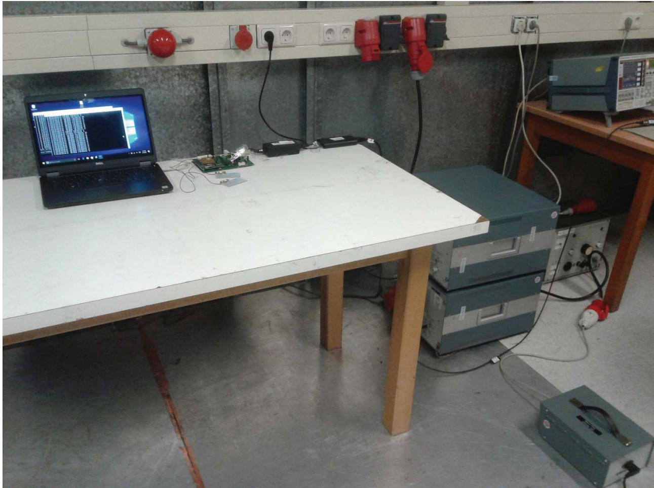
Photo 5: Photograph conducted emissions 0.15-30 MHz
