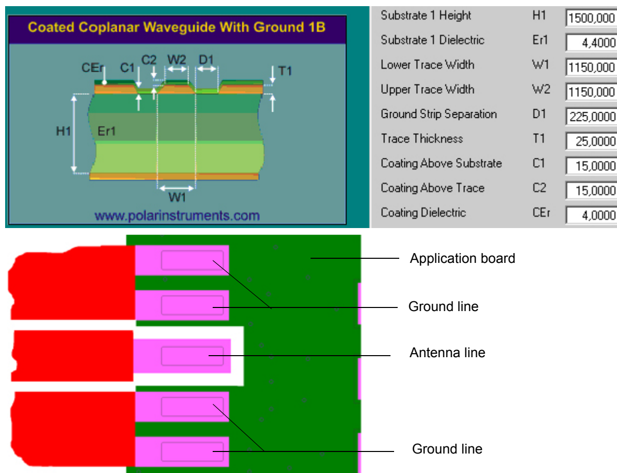
Figure 10: Micro-Stripline on 1.5mm Standard FR4 PCB - example 2
