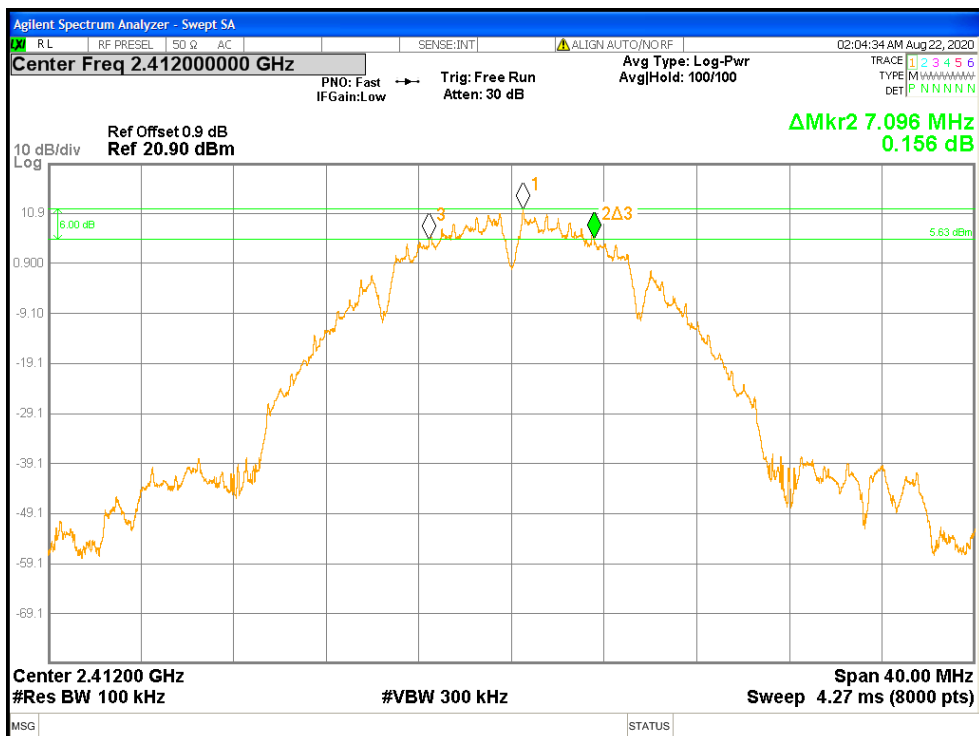
Figure 14: 6 dB Occupied Bandwidth-2412 MHz-802.11b-Ch0
