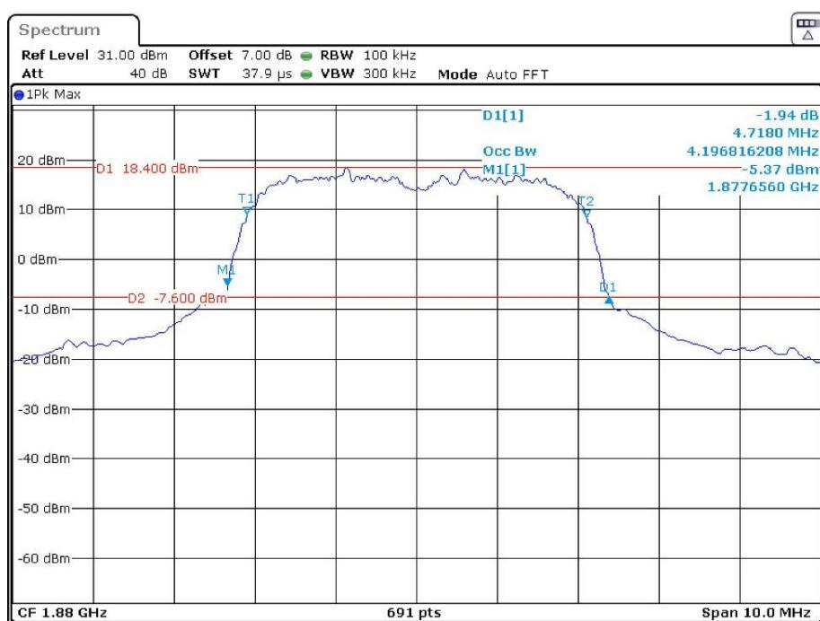
**26 dB Emissions &99% Occupied Bandwidth for HSDPA (16QAM) Mode, High channel**
