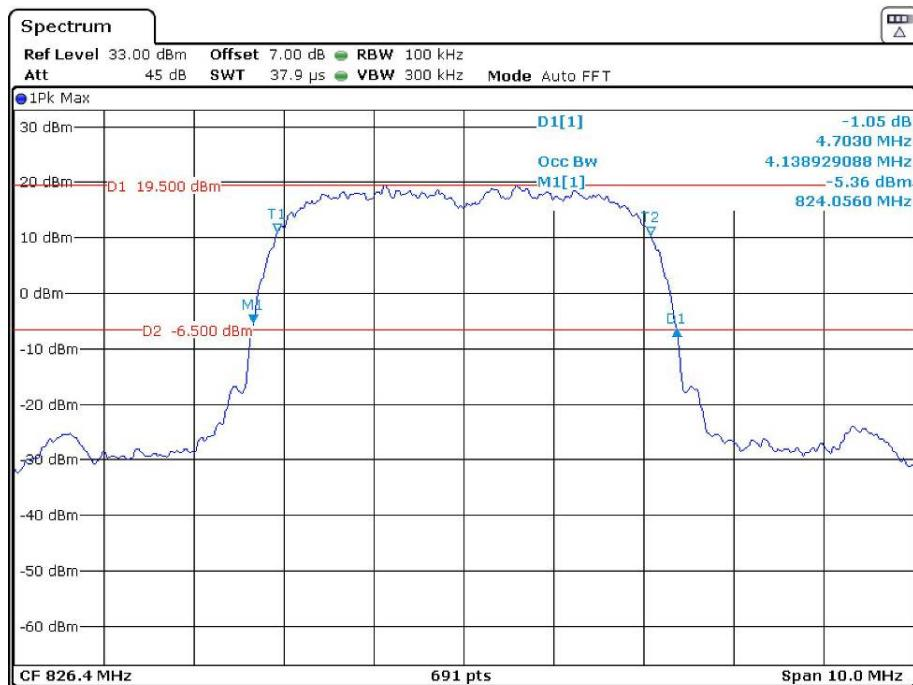
**26 dB Emissions & 99% Occupied Bandwidth for RMC (BPSK) Mode, Middle channel**
