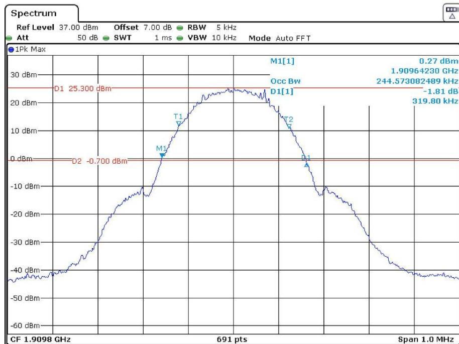
**26 dB Emissions &99% Occupied Bandwidth for EGPRS (8PSK) Mode, Low channel**
