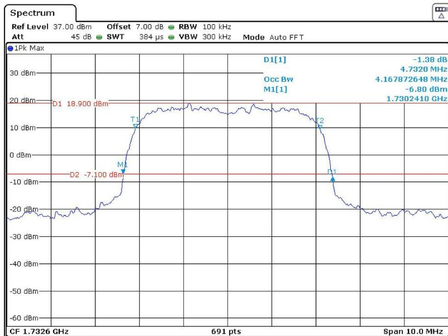
**26 dB Emissions &99% Occupied Bandwidth for HSUPA (BPSK) Mode, High channel**
