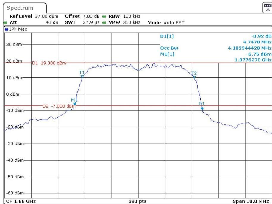
**26 dB Emissions &99% Occupied Bandwidth for HSUPA (BPSK) Mode, High channel**
