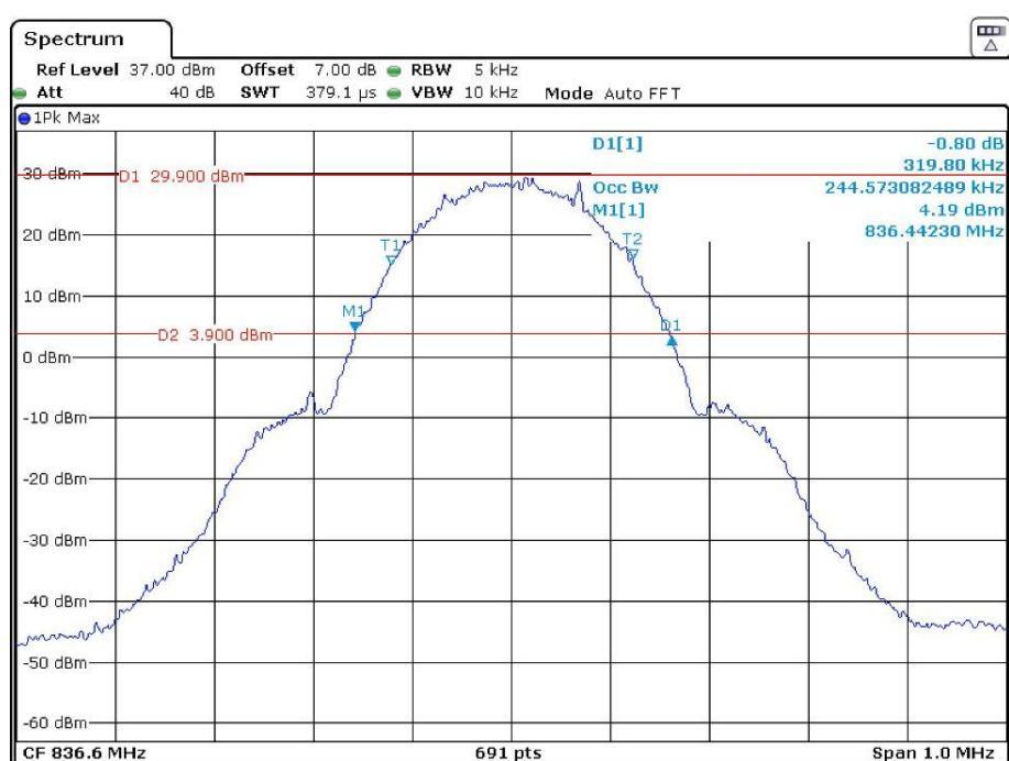
**26 dB Emissions &99% Occupied Bandwidth for GSM (GMSK) Mode, High channel**
