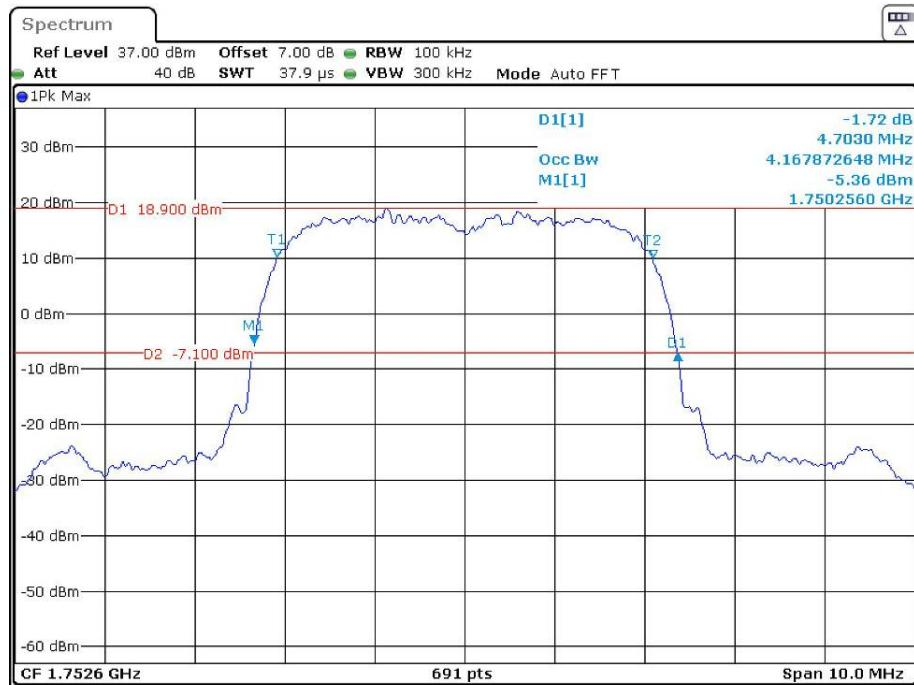
**26 dB Emissions & 99% Occupied Bandwidth for HSUPA (BPSK) Mode, Low channel**
