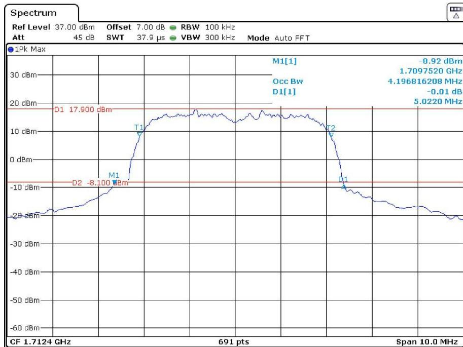
**26 dB Emissions &99% Occupied Bandwidth for HSDPA (16QAM) Mode, Middle channel**
