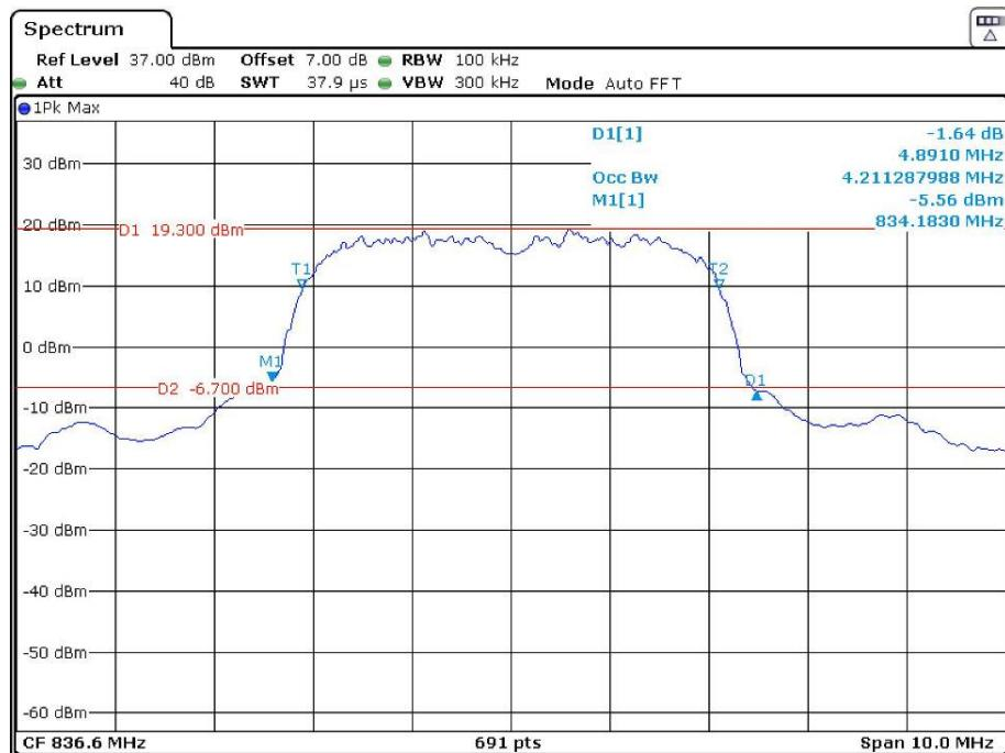
**26 dB Emissions &99% Occupied Bandwidth for HSUPA (BPSK) Mode, High channel**
