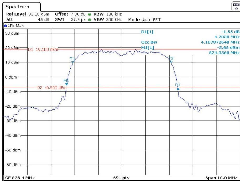
**26 dB Emissions &99% Occupied Bandwidth for HSDPA (16QAM) Mode, Middle channel**
