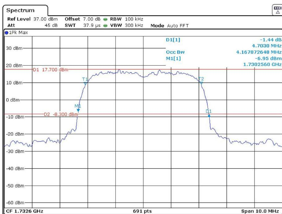
**26 dB Emissions &99% Occupied Bandwidth for HSDPA (16QAM) Mode, High channel**
