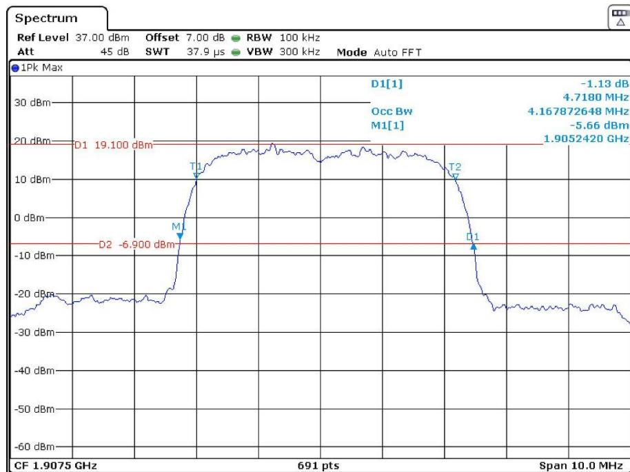
**26 dB Emissions & 99% Occupied Bandwidth for HSUPA (BPSK) Mode, Low channel**
