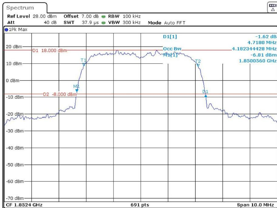
**26 dB Emissions &99% Occupied Bandwidth for HSDPA (16QAM) Mode, Middle channel**
