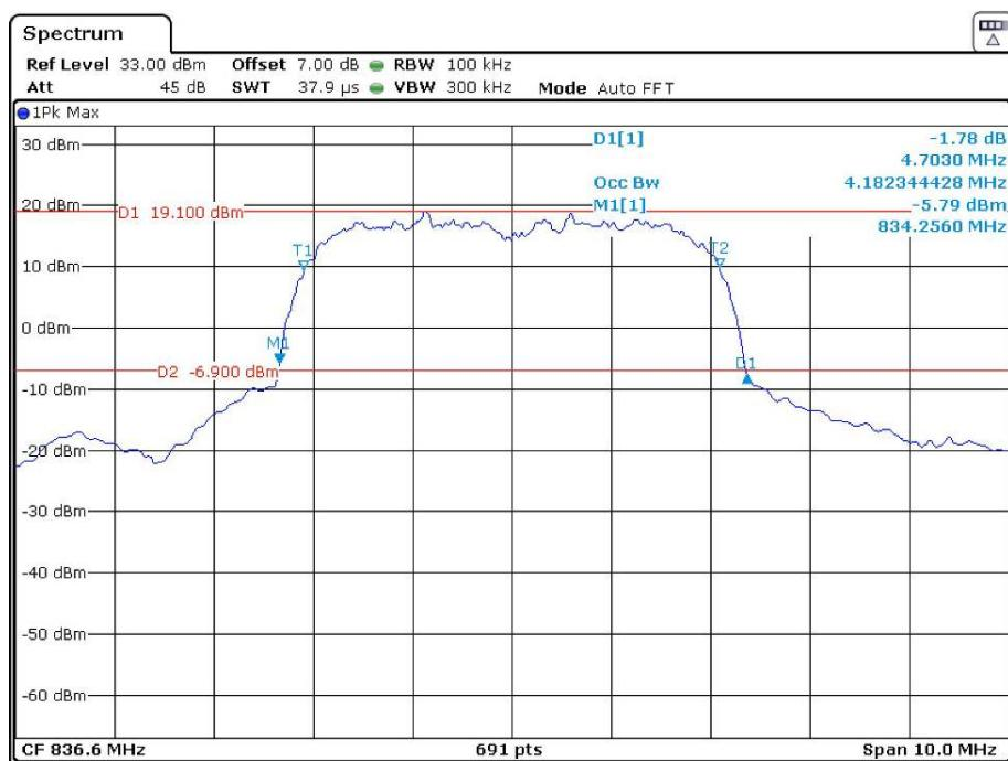
**26 dB Emissions &99% Occupied Bandwidth for HSDPA (16QAM) Mode, High channel**
