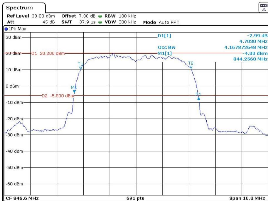
**26 dB Emissions & 99% Occupied Bandwidth for HSUPA (BPSK) Mode, Low channel**
