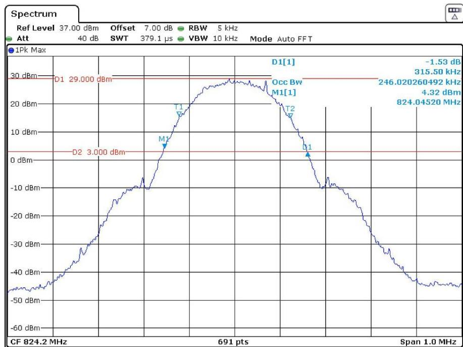
**26 dB Emissions &99% Occupied Bandwidth for GSM (GMSK) Mode, Middle channel**
