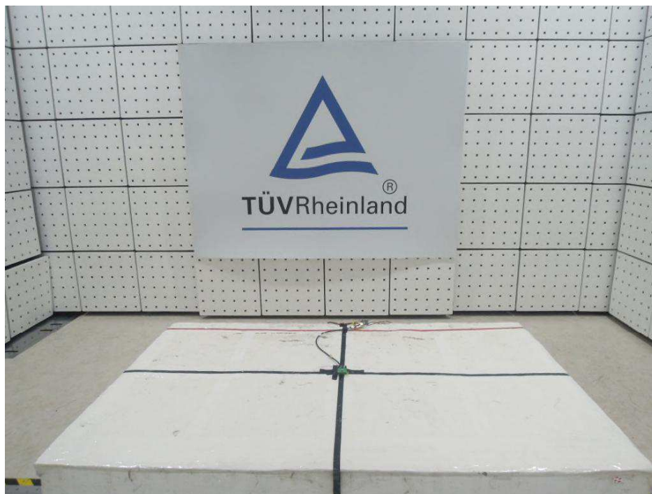
Photograph 1: Set-up for Spurious Emissions (Front View 1)
