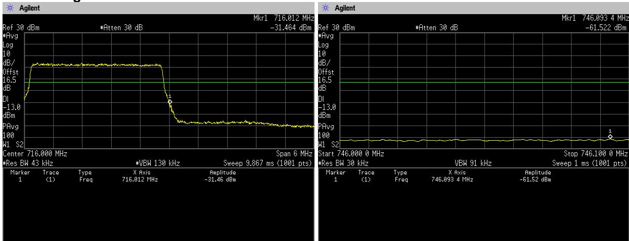
**QPSK, BW 5MHz, RB1-0****Channel: Low**
