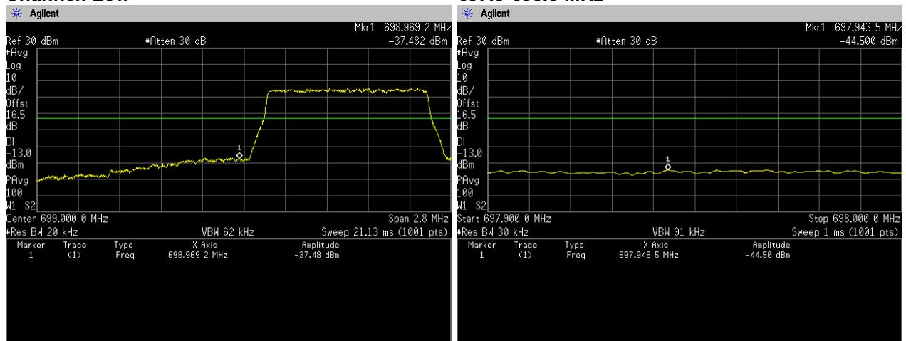
**16QAM, BW 1.4MHz, RB6-0****Channel: High**
