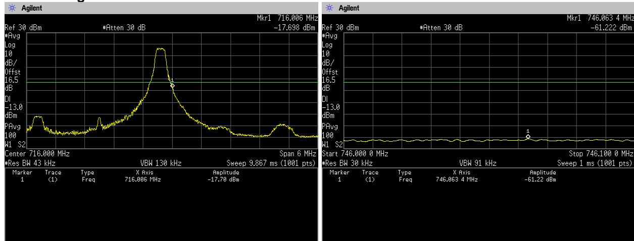
**16QAM, BW 3MHz, RB15-0****Channel: Low**
