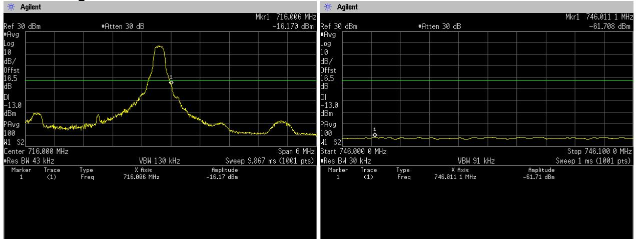
**QPSK, BW 3MHz, RB15-0****Channel: Low**
