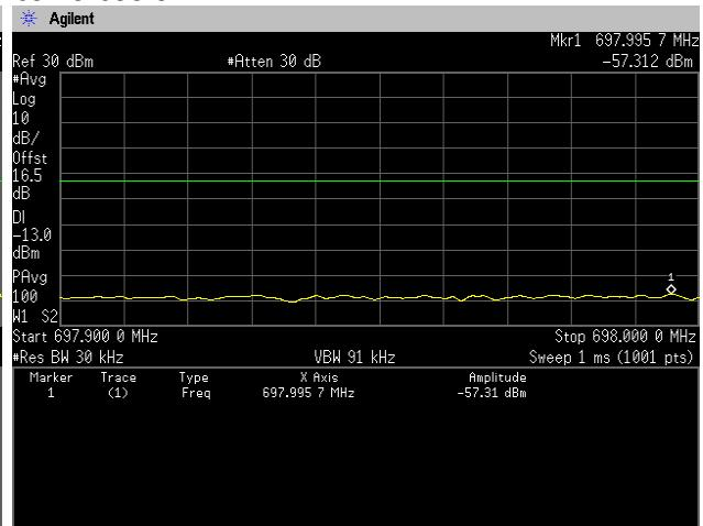
**64QAM, BW 1.4MHz, RB1-5****Channel: High**
